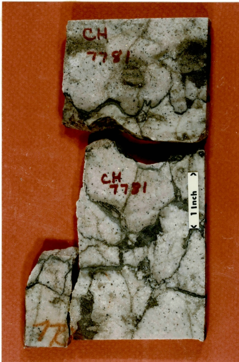
Figure 22. Carter Hester Core, -7,781 ft. Crinoidal packstone containing solution-enlarged fractures. Porosity has been occluded by cave muds, glauconite, and dolomite cement.
