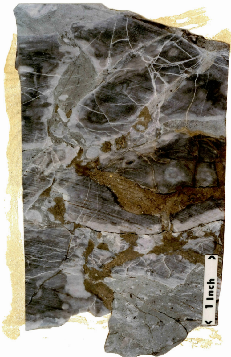
Figure 9. Cox Annis Core, -7,299 ft. Mosaic breccia. Chert clasts with dolomite and calcite cement. Pyritization a later event. Note interesting cross cutting relationships.
