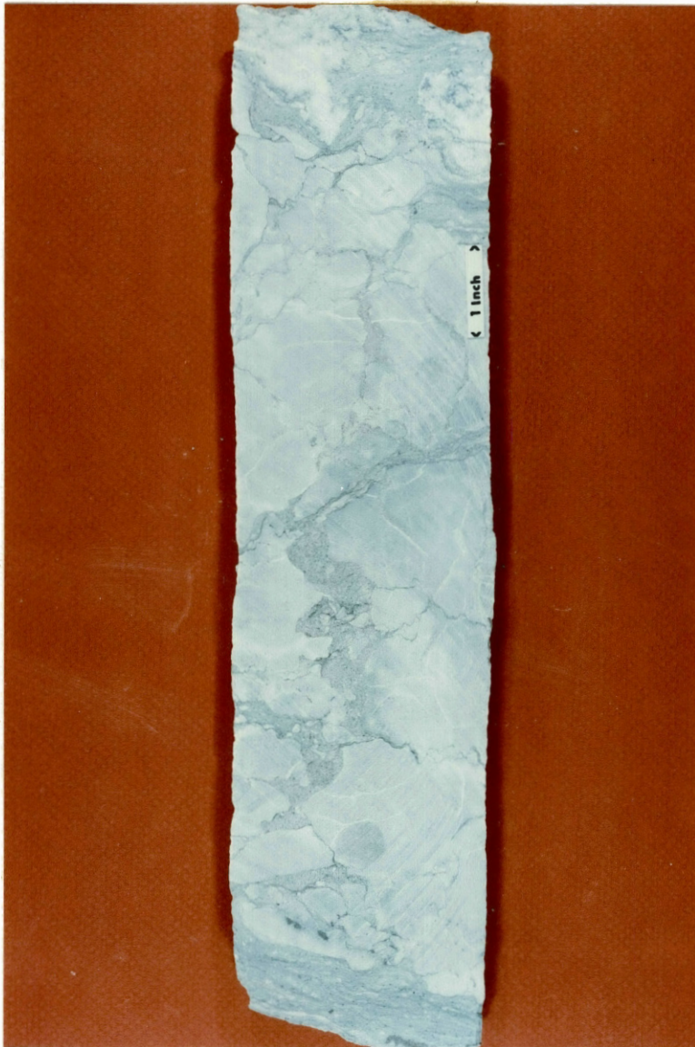
Figure 10. Pelto Cheatwood Core, -3,989 ft. Mosaic breccia, clast supported. Sediment between clasts contains glauconite, pyrite, quartz grains, and carbonate cement.
