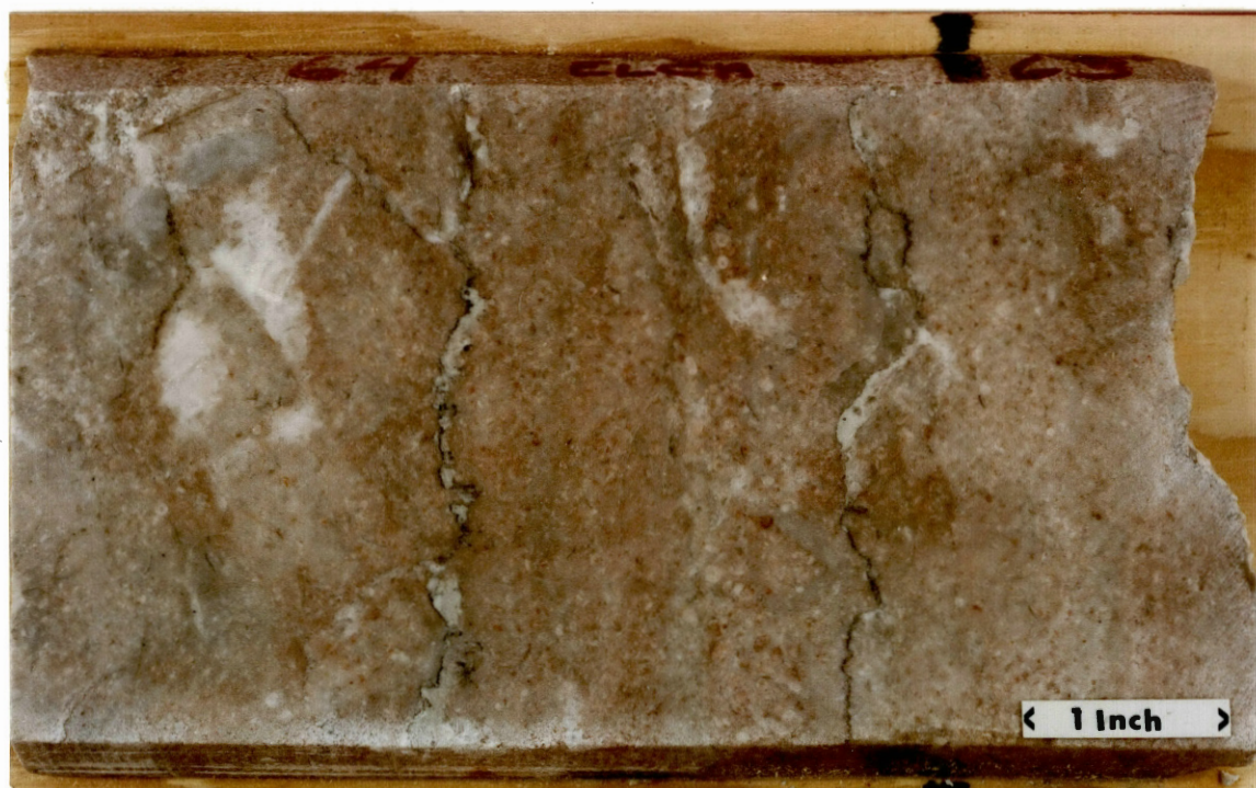
Figure 15. Cox Annis Core, -7,364 ft., and photomicrograph (X.N.), top of page. Packstone shoal facies with solution-enlarged vugs filled with clay-associated rhombic dolomite.
