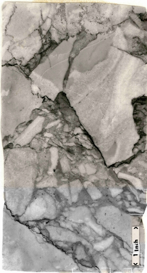
Figure 17. Cleary Kinney Core, -8,723 ft. Collapse breccia. Contains some fragments coated with calcite cement which appears to be flowstone.
