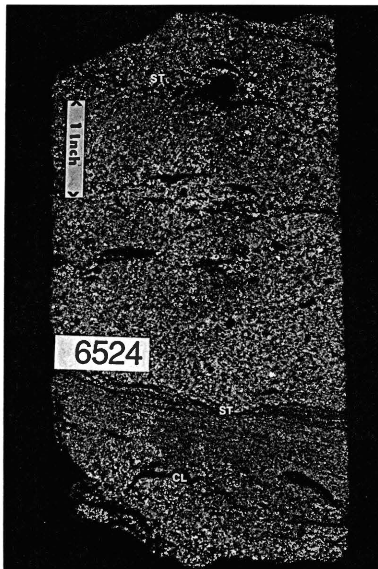
Figure 53. Photograph of Lower Morrowan sandstone typical of interval from 6526.7-6524 ft. in Shell Oil Co. No. 1-13 Finrock. Sample contains stylolites (ST) and clay rip-up clasts (CL).
