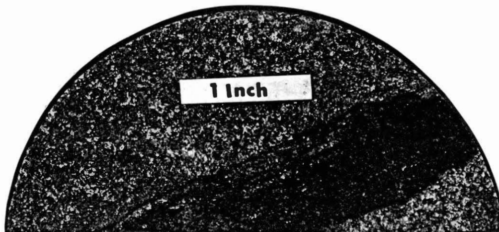
Figure 34. Carbonized plant remains in Upper Morrowan sandstone. Cities Service No. 4 Stonebraker "AN", 6272.8 ft.
