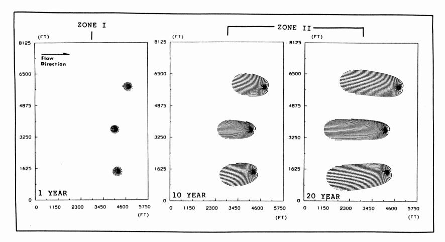
Figure 45. Results of the Delineation of Time-Related Wellhead Protection Areas for Edmond's Municipal Water Wells 44, 34, and 39 Using GPTRAC's Semi-Analytical Option
