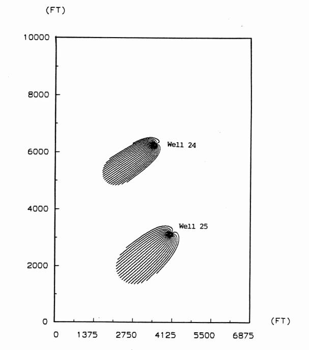
Figure 49. 10-Year Wellhead Protection Area Delineations for Edmond's Municipal Water Wells 24 and 25 Using GPTRAC's Semi-Analytical Option
