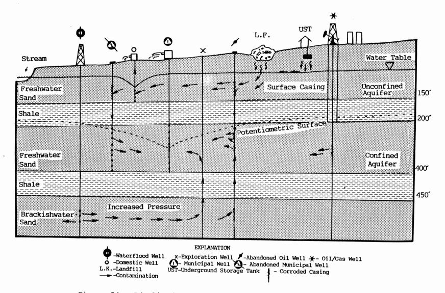
Figure 54. Idealized Cross-Section of the Central Oklahoma Aquifer Showing Some of the Potential Sources of Contamination Present in the Study Area
