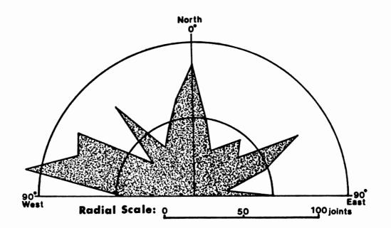
Figure 14. Rose Diagram Showing the Distribution of Fracture Orientations in the Central Oklahoma Aquifer near Guthrie, Oklahoma (Meyer, 1975)
