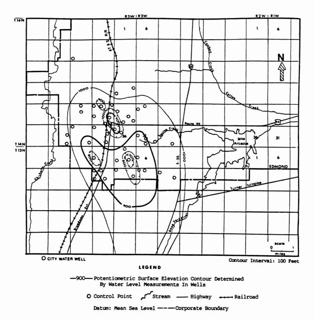
Figure 28. Static Water-Level Map for the Confined Portion of the Central Oklahoma Aquifer in the Study Area for August, 1989
