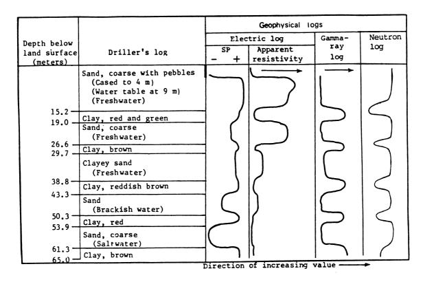
Figure 9. Responses of Various Well Logs to Different Lithologies (Heath, 1987).
