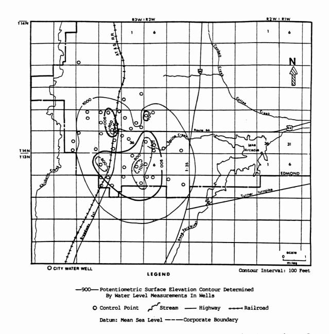
Figure 29. Static Water-Level Map for the Confined Portion of the Central Oklahoma Aquifer in the Study Area for February, 1989
