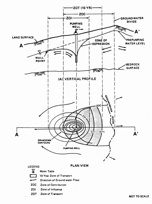
Figure 33. Terminology for Wellhead Protection Area Delineation (U.S. EPA, 1987 A)
