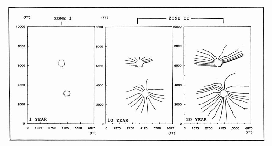
Figure 48. Results of the Delineation of Time-Related Wellhead Protection Areas for Edmond's Municipal Water Wells 24 and 25 Using GPTRAC's Numerical Option
