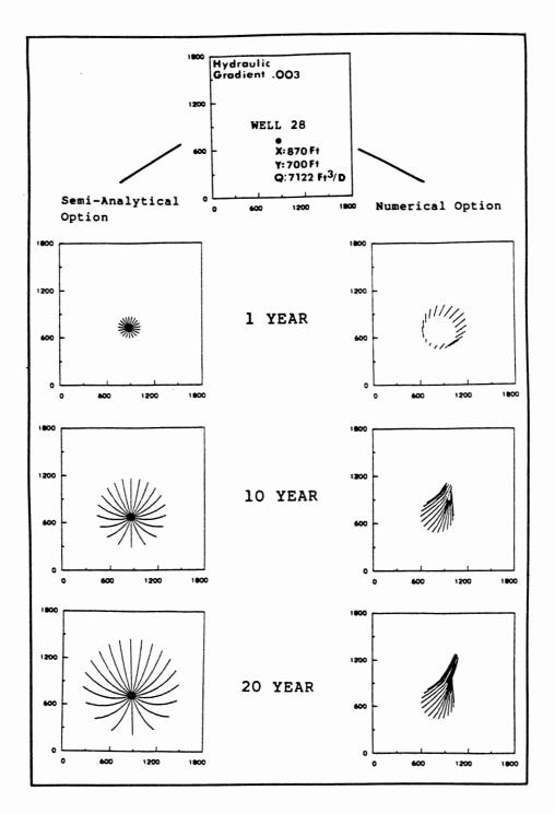
Figure 50. Comparison Between GRTRAC"S Semi-Analytical and Numerical Options in the Delineation of Time-Related Wellhead Protection Areas for Edmond's Municipal Water Well 28
