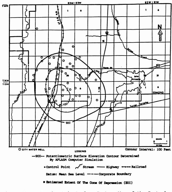
Figure 41. Potentiometric Surface Contour Map of the Central Oklahoma Aquifer in the Vicinity of the Edmond Well-field for the Month of August, 1990, Determined With APLASM
