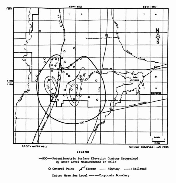
Figure 30. Pumping Water-Level Map for the Confined Portion of the Central Oklahoma Aquifer in the Study Area for August, 1990
