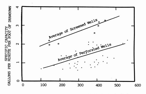
TOTAL INTERVAL PERFORATED OR SCREENED (IN FEET)
