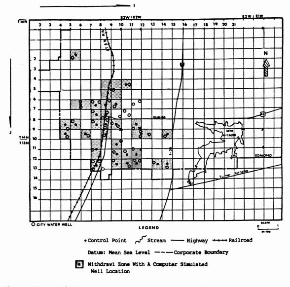
Figure 40. Grid Arrangement for the APLASM Simulation of the Drawdown of Edmond's Well-field
