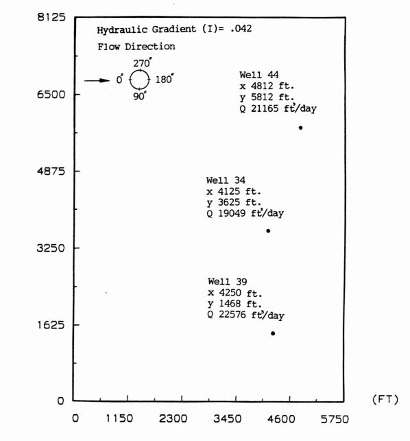
Figure 44. Area Setup for the Wellhead Protection Area Delineation for Edmond's Municipal Water Wells 44, 34, and 39 Using GPTRAC's Semi-Analytical Option
