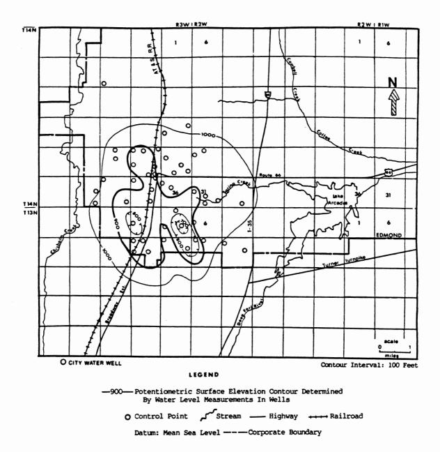
Figure 31. Static Water-Level Map for the Confined Portion of the Central Oklahoma Aquifer in the Study Area for August, 1990
