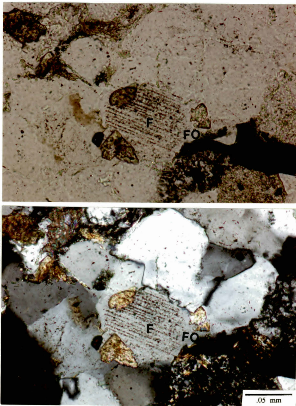
Figure 52. Feldspar (F) Overgrowth (FO) Recognized by Cleaner Outer Rim. Top PP. Bottom X-N. 20X. Southport Expl., Inc., Merrick No. 1-10, 13,948'7.5".
