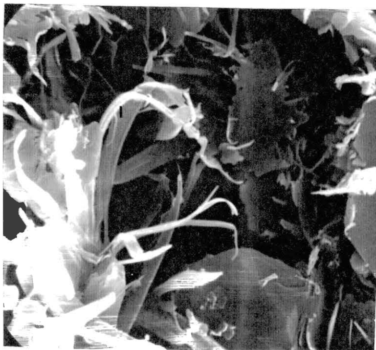
Figure 59. Scanning Electron Microscope Photograph From a Sample of the Louisiana Land & Expl. Gates No. 2-33 Core, 12,172'4". Illite (I) Lining Pores. 4300X.
