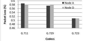
Fig. 25. Impact of the codec on the average percentage of packet loss.
