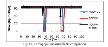
Experimental results show that AODVM-ALARM considerably improves the overall performance of real-time traffic in MANETs when link failures occur.
