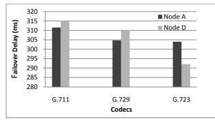
Fig. 23. Impact of the codec on the average Failover Delay.
