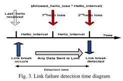
HELLO messages are broadcasted and utilized to detect broken links and maintain connectivity. Nodes are supposed to be receiving hello messages periodically to maintain connectivity.
