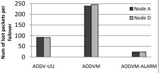
Fig. 16. Average failover loss in a two-way traffic scenario.
