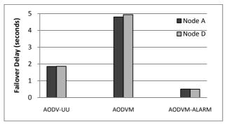
Fig. 15. Comparison of the average failover delay in a two-way traffic scenario.
