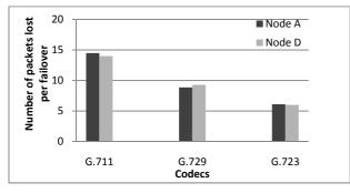
Fig. 24. Impact of the codec on the average number of packets lost.
