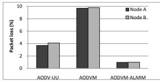
Fig. 17. Average percentage of packet loss per trial in a two-way traffic scenario.
