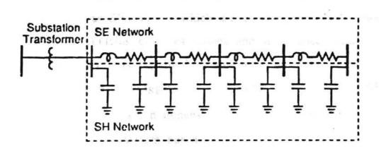
Figure 17. Distribution network decomposed into SE and SH networks. [5]
