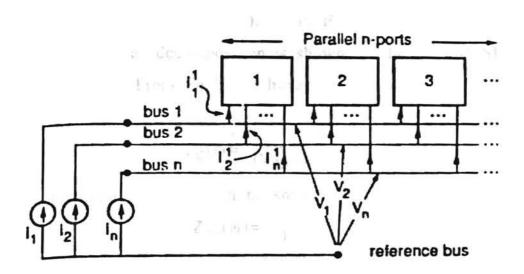
Figure 18. Parallel n-port circuits [5]
