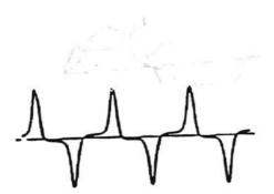
Figure 8. Typical Transformer Magnetizing Current [17]
