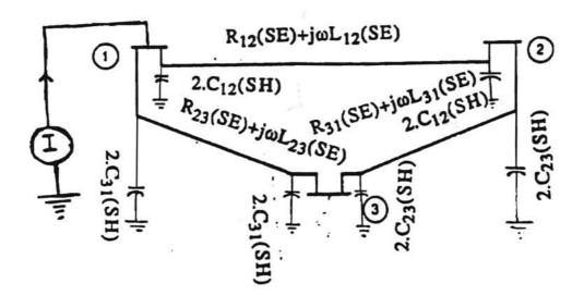
Figure 21. Three bus power system
