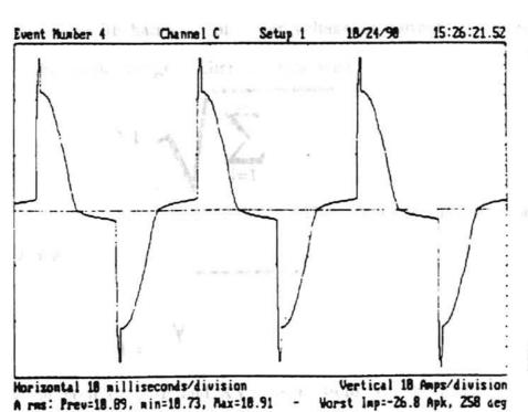
Figure 13. Waveform of SCR-Controlled Load [15]
