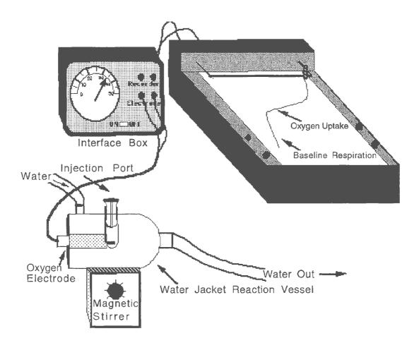
functioning properly. The oxygen permeable membrane covering the electrode was replaced when necessary. <u>Chart Parameters.</u> The chart was set to move one inch every 30 minutes.
