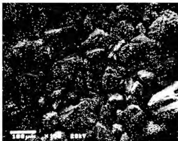
SEM photographs of solids obtained from the underflow of the hydrocyclone of sample treated with dispersant and dispersator (11385-58). (A) x150 image showing particle morphologies. (B) x500 image showing detailed particle morphologies. (C) x150 image showing barium X-ray map of image shown in (A). (D) x500 image showing barium X-ray map of image shown in (B).
