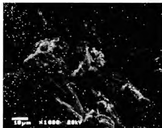
SEM photographs of sample 11374-80. (A) x250 image showing particle morphologies. (B) x1000 image showing detailed particle morphologies. (C) x250 image showing barium X-ray map of image shown in (A). (D) x1000 image showing barium X-ray map of image shown in (B).
