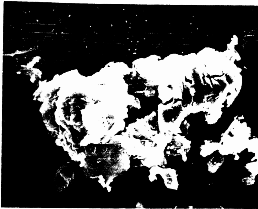
Figure 5.21. An SEM micrograph of a chip that appears highly stressed formed at 0.2 N load
