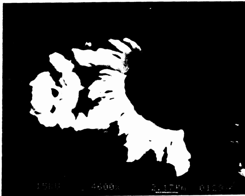
Figure 5.22. SEM micrograph of a brittle chip formed at 0.2 N load
