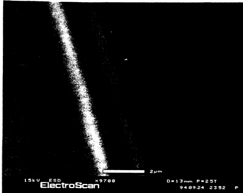
Figure 5.3. SEM micrograph showing smooth groove produced in the in-situ scratching mode (Load:0.035 N and Scratching Speed:0.143 mm/sec)
