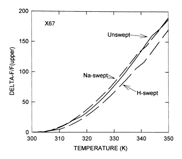
Figure 11. Frequency versus Temperature for X-67 resonators for temperature range 300K to 350K.
