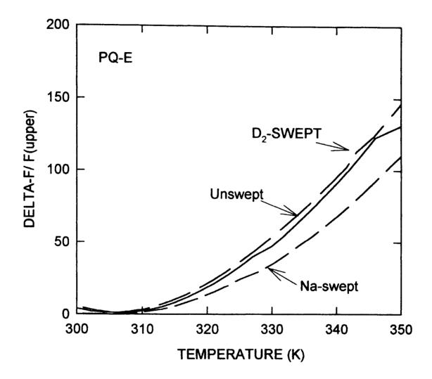
Figure 6. Frequency versus Temperature for PQ-E resonators for temperature range 300k to 350K.
