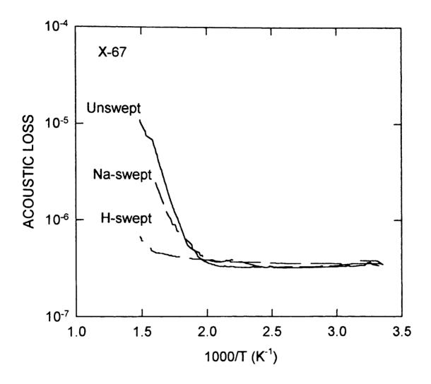
Figure 8. Acoustic Loss versus 1000/T(K) for X-67 unswept, H-swept and Na-swept resonators.
