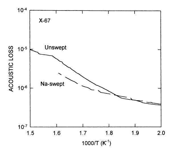
Figure 9. Acoustic Loss versus 1000/T(K) for X-67 unswept and Na-swept resonators.
