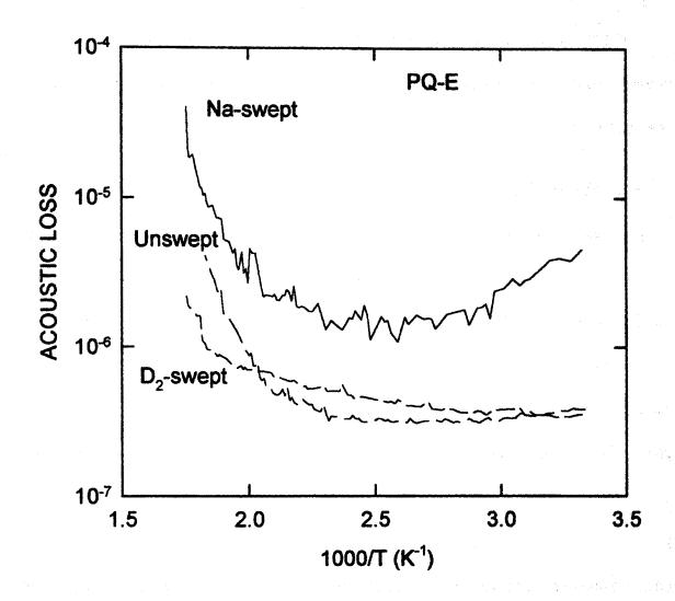
Figure 3. Acoustic Loss versus 1000/T(K) for PQ-E unswept, Na-swept and D<sub>2</sub>-swept resonators.
