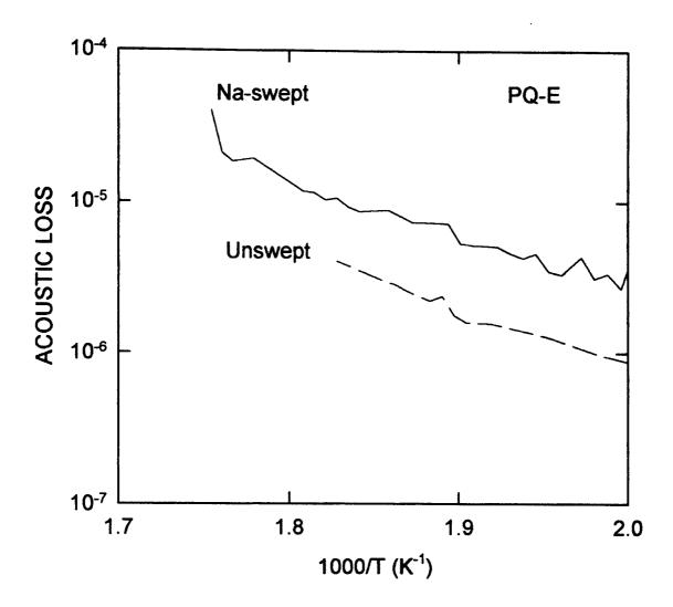
Figure 4. Acoustic Loss versus 1000/T(K) for PQ-E unswept and Na-swept resonators.
