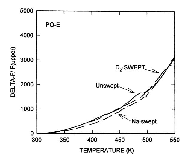
Figure 5. Frequency versus Temperature for PQ-E unswept, Na-swept and D<sub>2</sub>-swept resonators.
