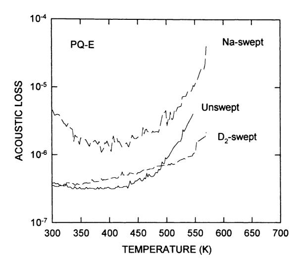
Figure 2. Acoustic Loss versus Temperature for PQ-E unswept, Na-swept and D<sub>2</sub>-swept resonators.
