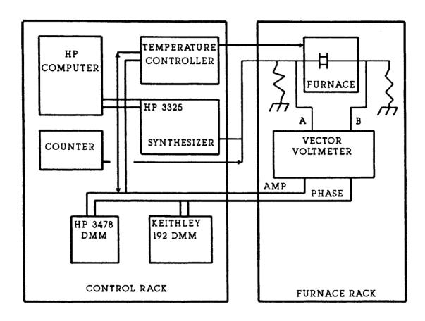
Figure 1. Block diagram for transmission technique for the measurement of acoustic loss.
