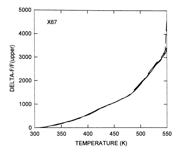
Figure 10. Friequency versus Temperature for X-67 unswept, H-swept and Na-swept resonators.
