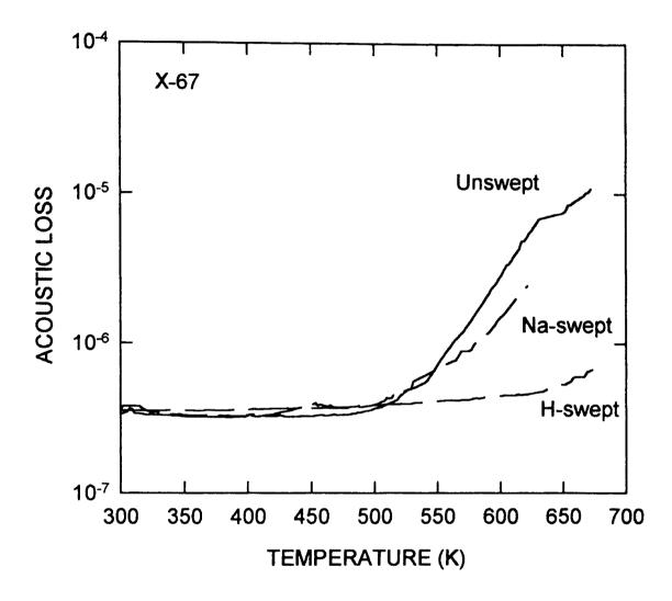
Figure 7. Acoustic Loss versus Temperature for X-67 unswept, H-swept and Na-swept resonators.
