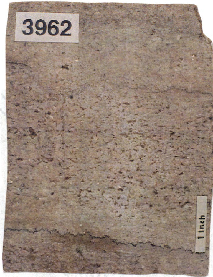
Figure 9. Viola Springs grainstone depth interval 3962 with high porosity. Abundant fossils of bryozoan, brachiopod and echinoderms.
