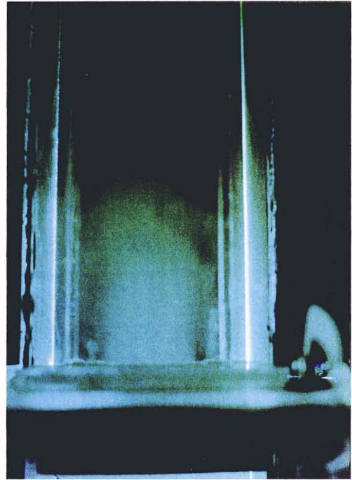
Fig. 4.55 Flow Visualization Using Water Mist Upstream of the Filter
