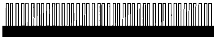
Figure 2.1 The top and side views of the Purolator AF3192 filter. The pleats are 3 cm high with a 3 mm pitch. The media is about 635\mu\text{m} thick.
