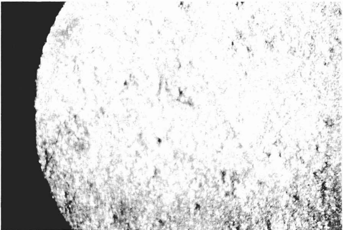
Fig 29: Top surface of specimen in Fig 28, after chemical cleaning showing uniform pitting all over the surface
