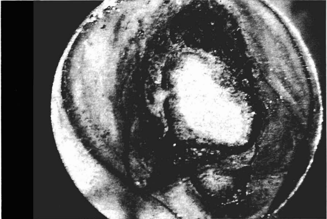
Fig 42: Cylindrical specimen of GCI showing crevice corrosion after immersion in environol for 4 weeks.
