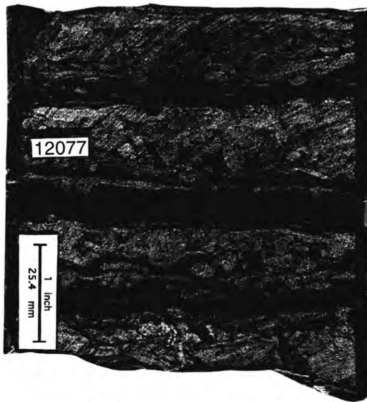
Figure 47. Core Sample from the Midwest Booth Exhibiting Burrowing Associated with the Delta Facies.
