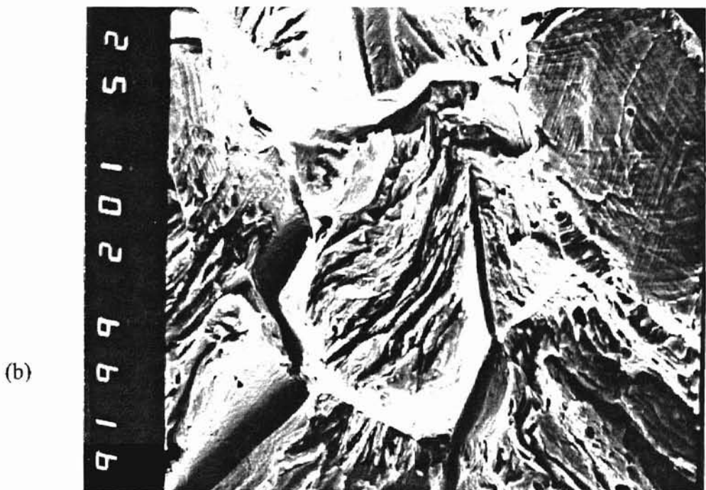
Figure 28. As-received specimen broken in mercury. (a) General specimen view, 20\times . Note MVC smooth region, lower left. (b) Detail, 1000\times . Note cleaved slip bands as well as some prominent slip bands on the sheared grain at the upper right.
