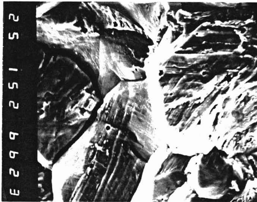
Figure 29, continued. (c) Detail, showing TG + IG mixed-mode cracking, 500\times . This particular zone has an unusually high amount of IG contribution. (d) Detail of (c), 1500\times . IG region; note slip on three systems, secondary cracking.
