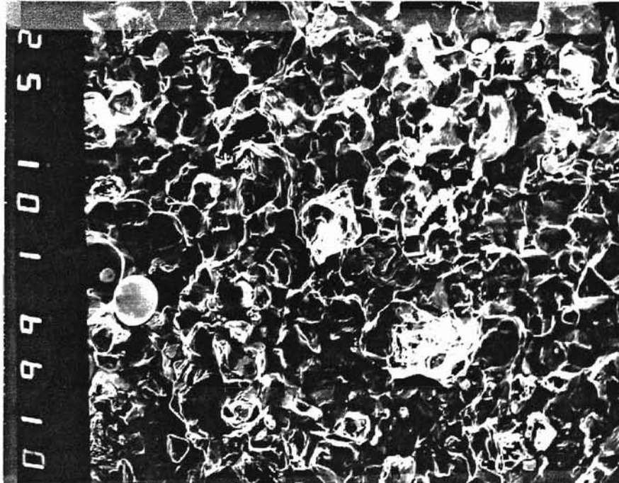
Figure 26. Unwetting drops of mercury on (a) 600-grit polished surface (SZM) and (b) fracture surface (SEM, 100 \times ).
