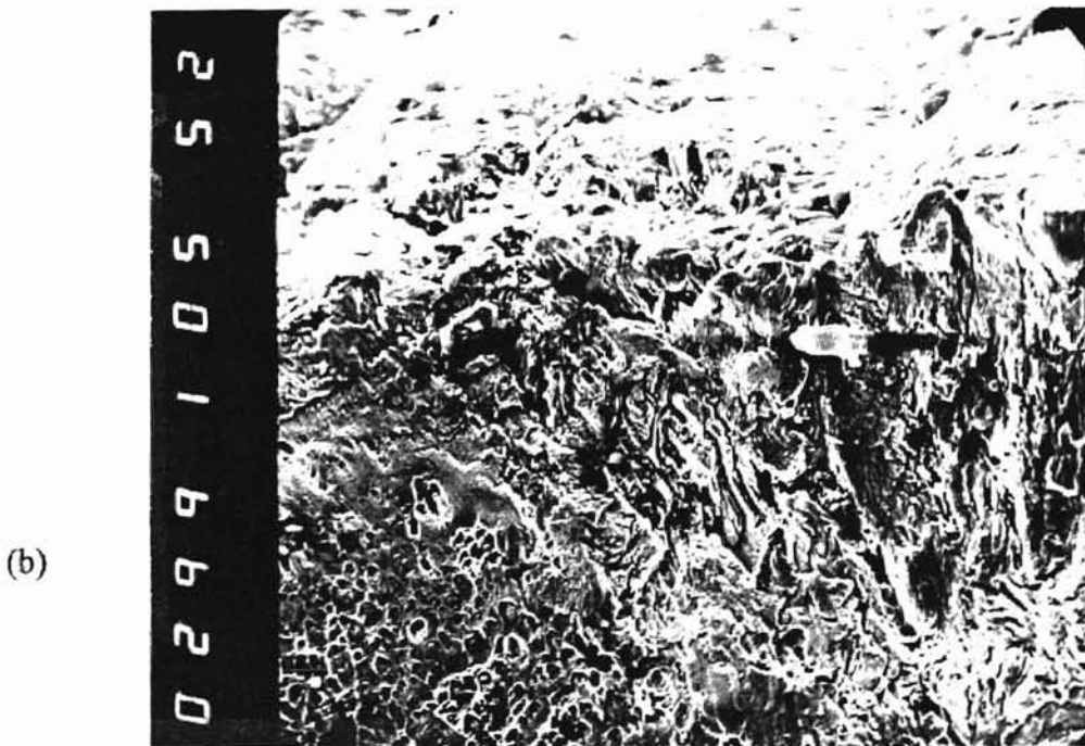
Figure 34. Fracture surface of annealed and cold-worked (to 70% of the tensile strength) specimen. (a) General view, 20 \times . (b) Detail, from 12 o'clock, showing TG origin zone and transition to MVC, 500 \times .
