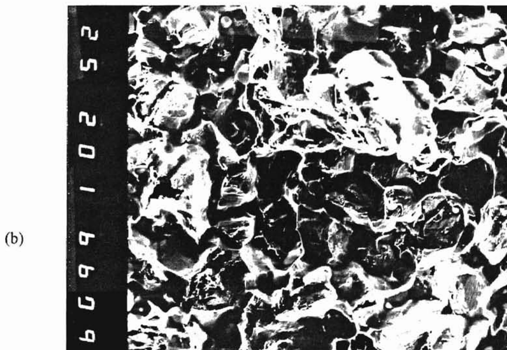
Figure 31. Fracture surface of sensitized specimen broken in mercury. (a) General specimen view, 20 \times . (b) Detail, 200 \times .
