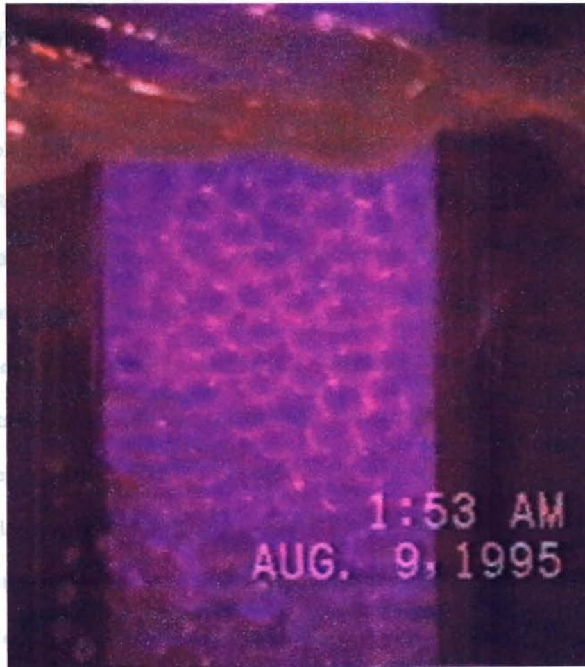
Figure 5. Plasma In The Presence Of Glass Beads -- This picture is from data set #89 where air flows through the annulus of reactor B. The smudge across the top of the picture is the silicon that holds the outer electrode container together.
