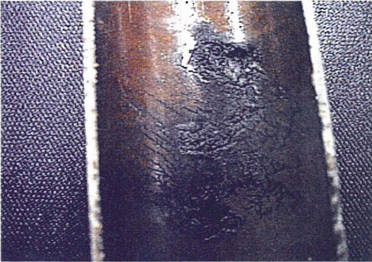
Figure 7c. Electrical breakdown of glass-filled phenolic resin (inner surface of the outer dielectric)
