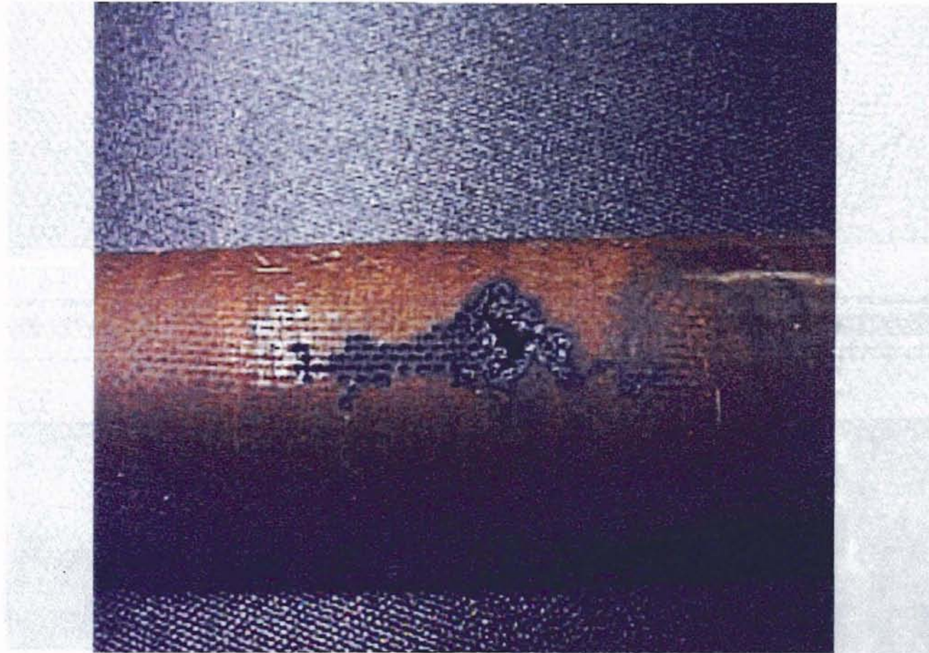
Figure 7b. Electrical breakdown of glass-filled phenolic resin (outer surface of the outer dielectric)
