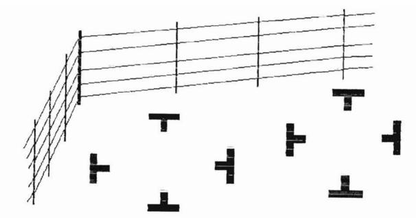
Fig. 3. Wooden T orientation and configuration for 25 groups of four T's anchored inside the 20-ha electricfence predator exclosure at Salt Plains National Wildlife Refuge, Oklahoma, in 1996.
