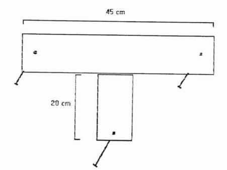
Fig. 2. Wooden T dimensions constructed to provide 2-90 degree corners for potential least tern nest sites and location of nails to anchor T's on the alkaline flat inside electric-fence predator exclosures at Salt Plains National Wildlife Refuge, Oklahoma, in 1995 and 1996.
