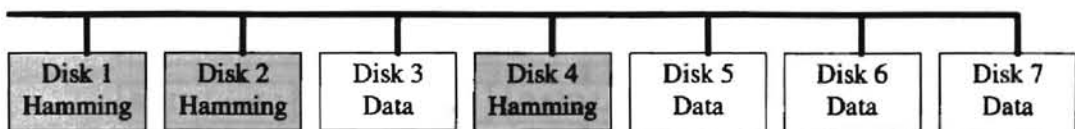
Figure 2-7 RAID level 2 as Hamming Coded disk array.
