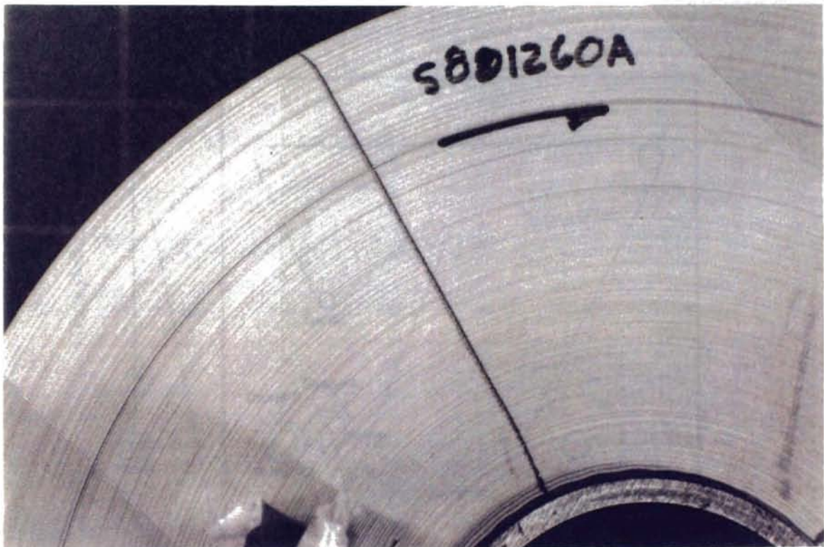
Figure 17: J-Line for a High Nip Load Winding Condition
