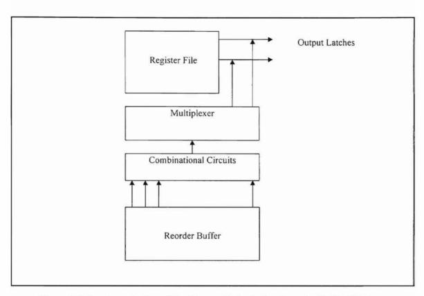
Figure 5.8 Implementation of the Bypass Paths in the Reorder Buffer Strategy
