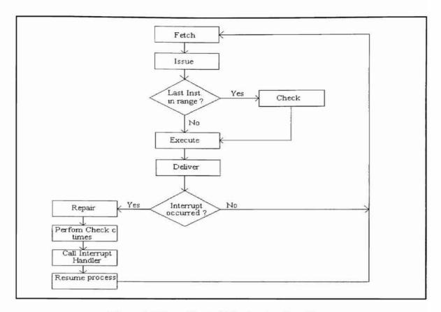
Figure 4.1 Flow Chart of Checkpoint Algorithm
