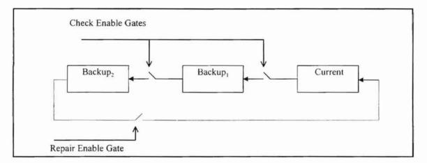
Figure 4.12 Physical implementation of Logical Spaces and the associated data paths
