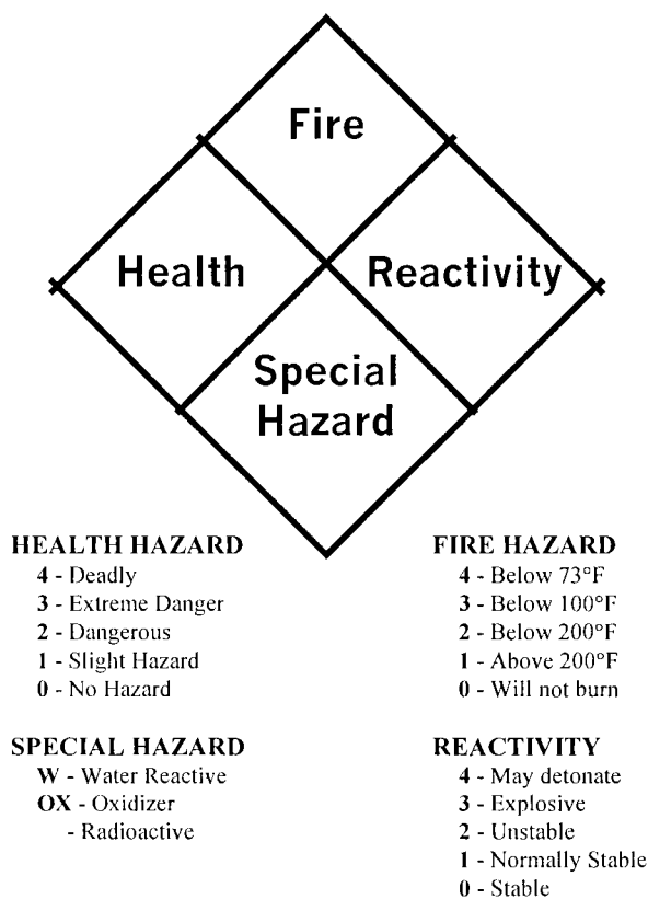
Figure 3. The NFPA 704 Marking System
