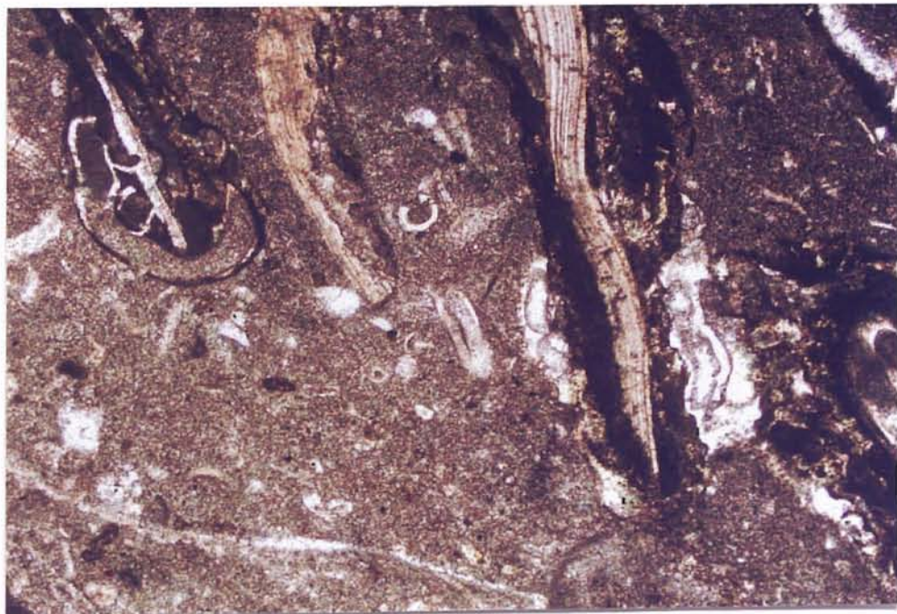
Photograph 112, SK-38, Crouse Limestone, Unit: 3 wackestone, brachiopod, oncolid, micrite,
