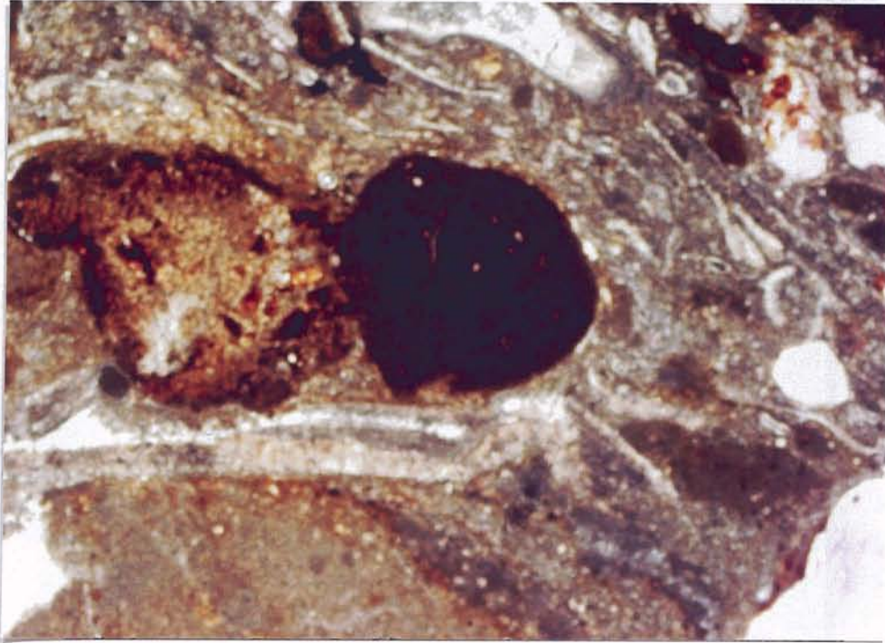
Photograph 31, NK#1, Crouse Limestone, Unit: 1 packstone, intraclast, trilobite, ostracode, micrite.
