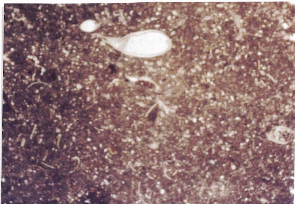
Photograph 44, NK#1, Speiser Shale, Unit: 4 wackestone, peloid, ostracode, micrite.
