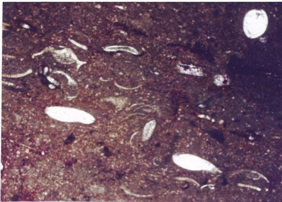
Photograph 34, NK#1, Crouse Limestone, Unit: 15 wackstone, ostracode, micrite hematitic.
