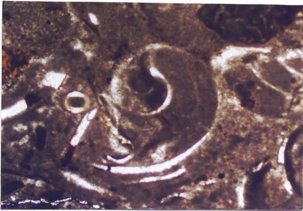
Photograph 111, SK-38, Crouse Limestone, Unit: 1 packstone, gastropod, bioclast, micrite.
