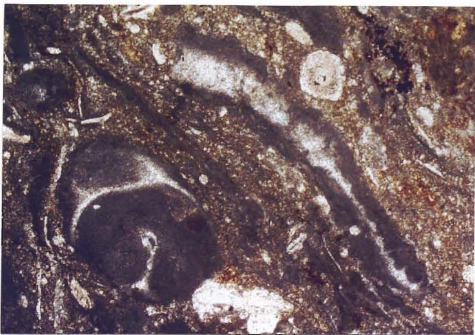
Photograph 115, SK-38, Crouse Limestone, Unit: 9 wackestone, oncoïd, echinoderm, bioclast, algae.
