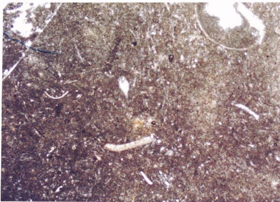
Photograph 148, SK-166, Funston Limestone, Unit: 22 mudstone, ostracode, bioclast, micrite.
