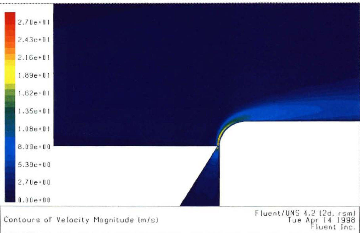
Figure 3.8 Contours of velocity magnitude showing jet attachment ( b = 0.03'' , R = 0.141'' , h = 0'' , P = 0.15 psi)
