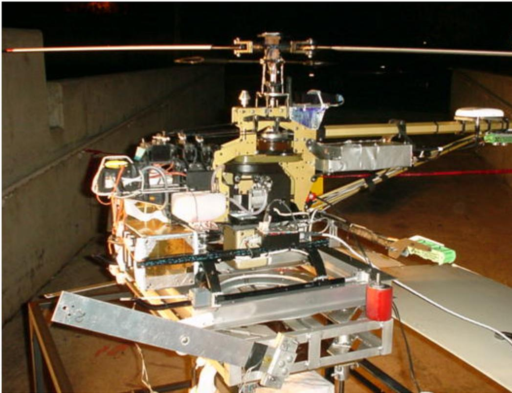
Figure K.3: Torque Experiment with Helicopter on the HTF with cantilever beam as a torque measuring device.
