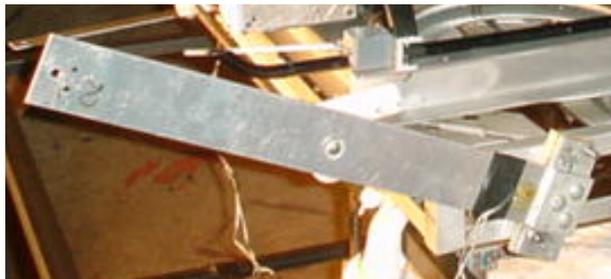
Figure I.18: Cantilever Beam with strain gages.
