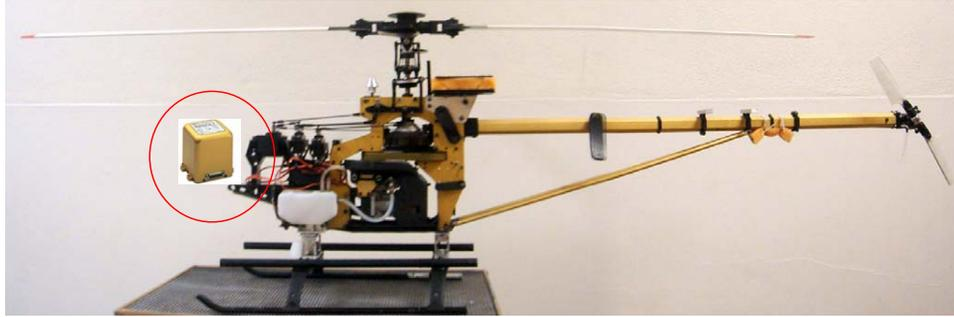
Figure 6.1: MontionPak Sensor Suite Location at front of the Helicopter.
