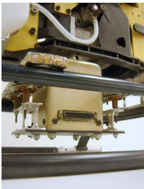
Figure 6.5: MontionPak Sensor Suite mounted on vibration isolation pads and positioned beneath the helicopter engine.
