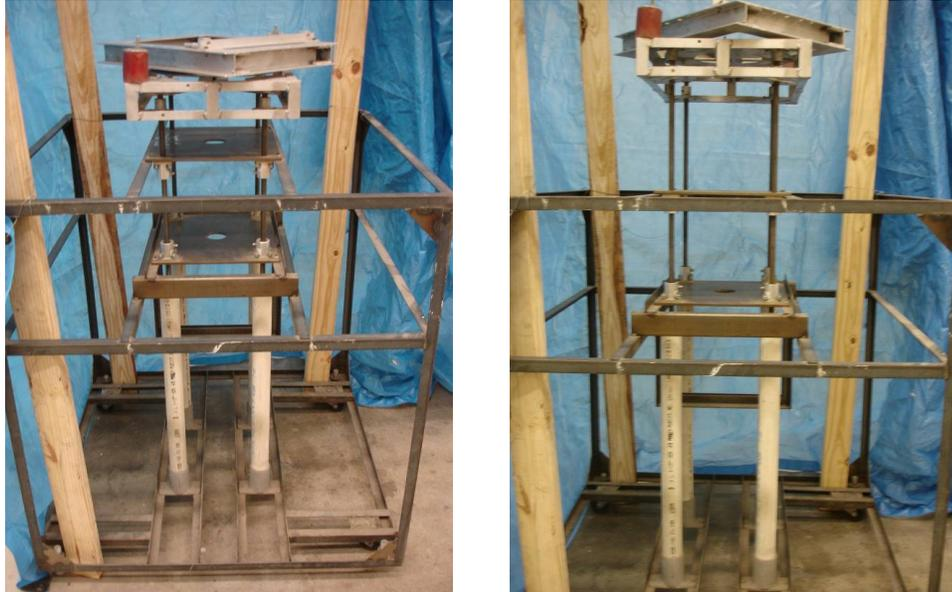
Figure 4.1: Side view of the LDTS. Note that in the left picture the altitude stand is at its minimum point. On the right, the attachment plate is at its maximum height of 14 in (0.36 m).
