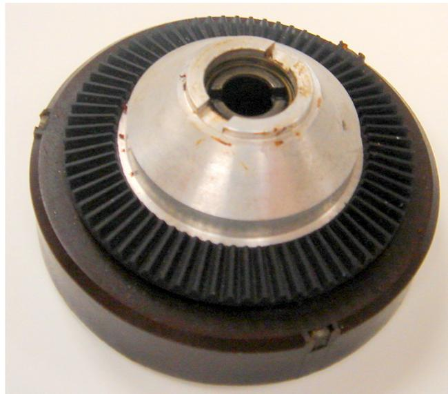
Figure 2.15: Main Rotor Gear with Embedded Permanent Magnets
