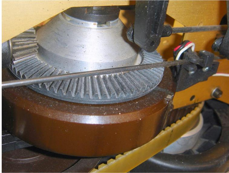
Figure 2.16: Hall Effect Sensor near the Main Rotor Gear with Embedded Permanent Magnet
