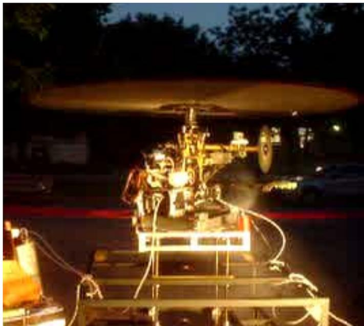
Figure 10.2: Helicopter on the Linear and Directional Test Stand (LDTS) during a real-time yaw rate experiment.
