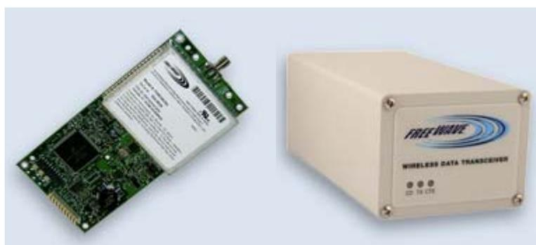
Figure I.5: FreeWave Wireless Data Transceiver On-Board Card and Ground Station Unit.
