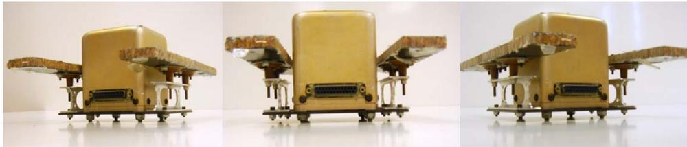
Figure 6.4: Photo montage of the MontionPak Sensor Suite mounted on vibration isolation pads.
