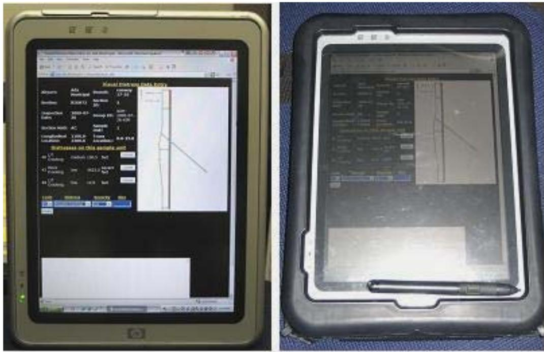
Figure 2-11: Hewlett Packard's tablet PC tc1100 used for real-time pavement condition entry
