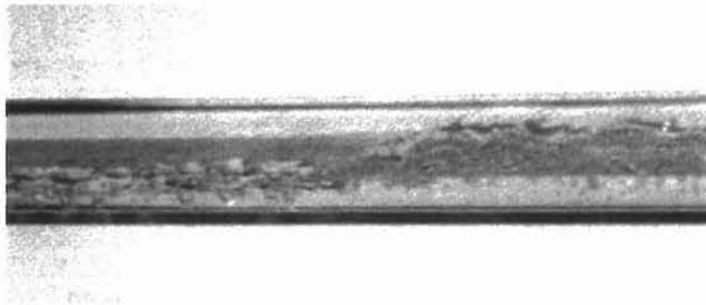
Photograph 3.3: Stratified/Slug Transition Water: 3.43 gpm (12.99 lpm)/Air: 10.8 gpm (40.88 lpm)
