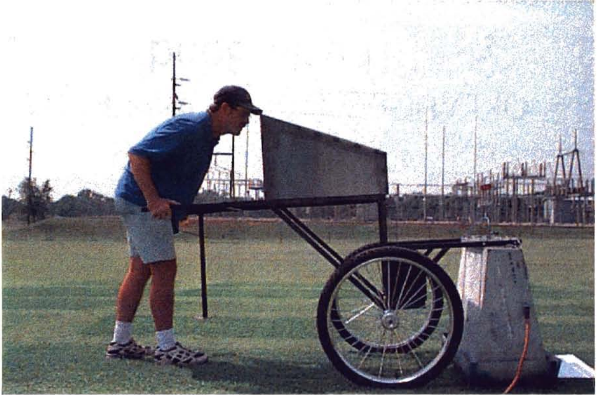
Figure 2. Apparatus for obtaining turf reflectance showing shielded computer compartment (upper portion being viewed by operator) and artificial light hood (light source and shield resting on turf)
