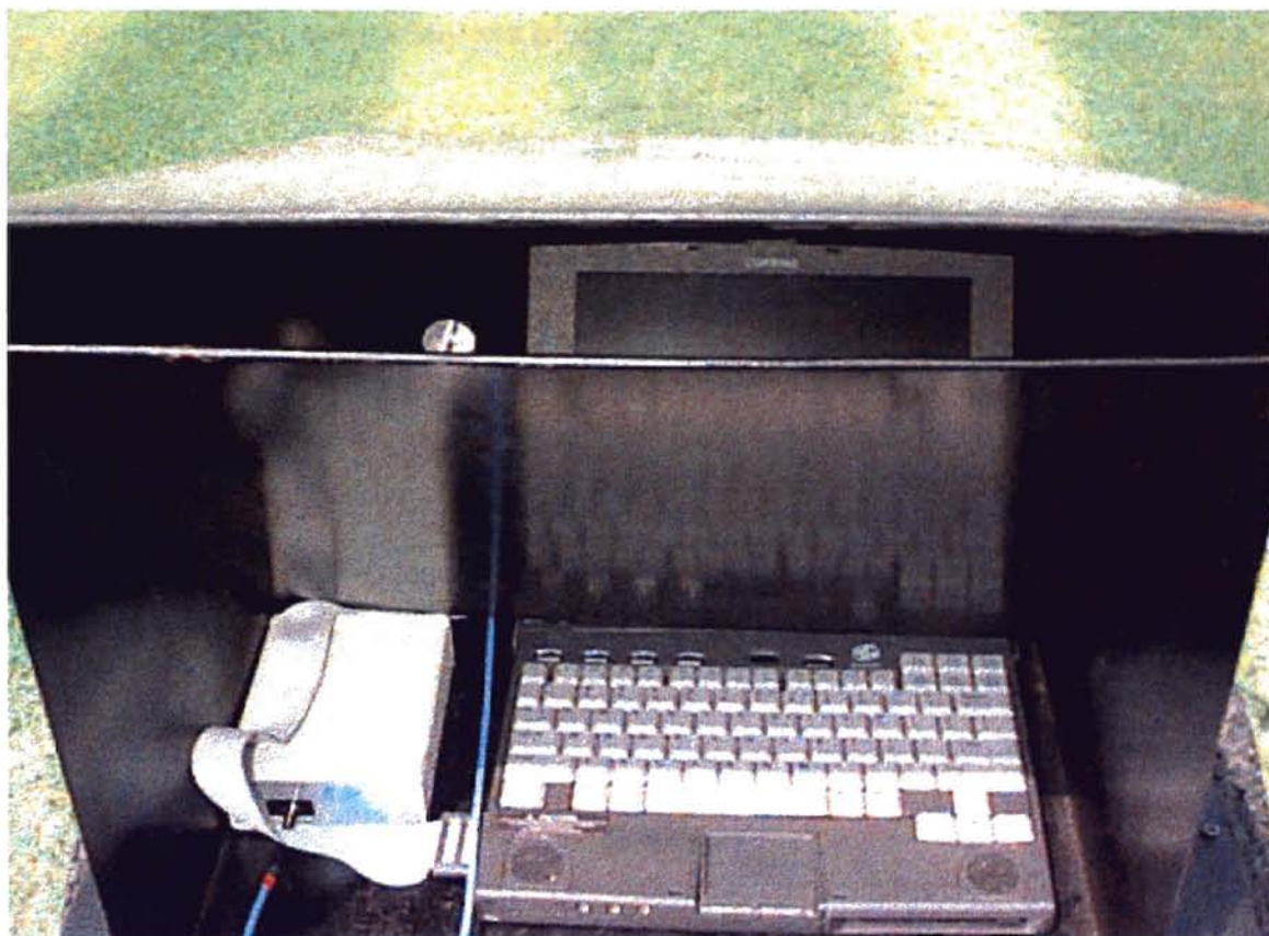
Figure 3. Laptop computer and S2000 spectrometer inside viewing hood.
