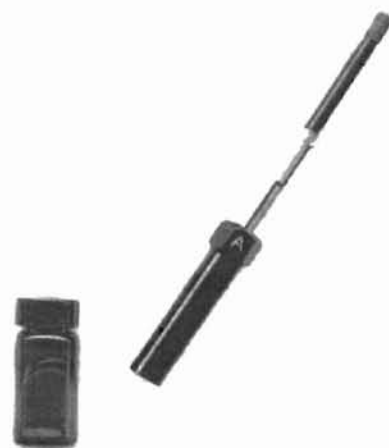
Fig 2 - Solid phase micro-extraction fiber assembly with sample vial and magnetic stir bar.
