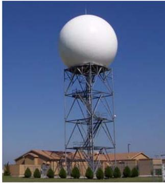
Figure 4.1. Dual polarization Doppler research radar KOUN in Norman, OK
