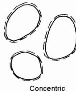
Figure 40. Clay distribution patterns (after Wilson and Pittman, 1977) and types of dispersed clay in a sandstone reservoir.
