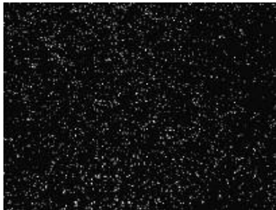
Figure 2.9 Double pulsed particle image (courtesy of Dantec Dynamics.com)
