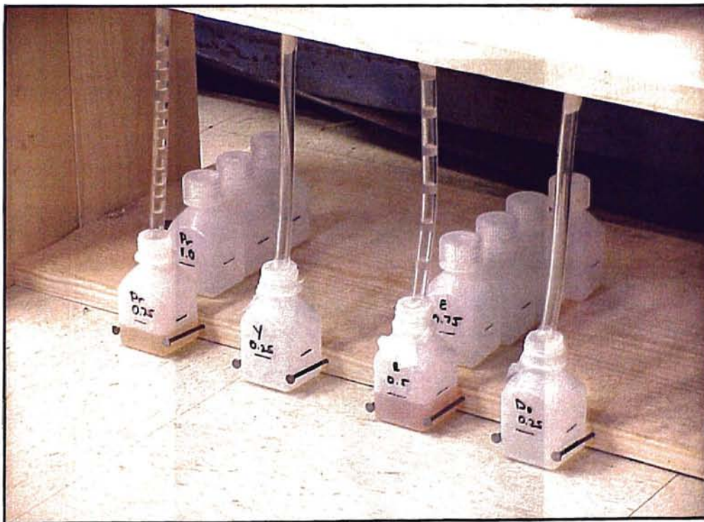
Figure II-1c. Leachate collection bottles for coarse textured soils.
