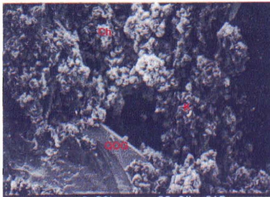
Figure 50. RMU #13 Well. Sample Depth: 5031.8 ft. SEM Photomicrograph. QOG= quartz overgrowth, K= kaolinite, Ch= chlorite
