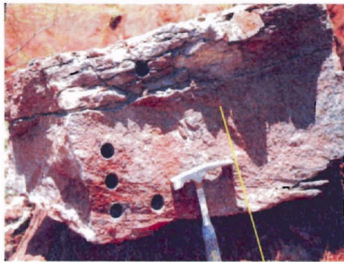
Lens # 2: Carbonate cemented, erosive base, cross-bedded, overlain by ripple-laminated, very fine grained sandstone.
