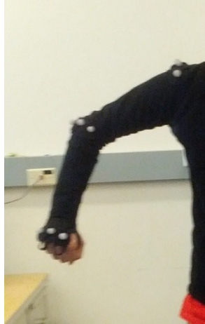
Figure 30 - Twelve markers attached to right hand finger tip, elbow and shoulder for detection by the VICON motion capture system
