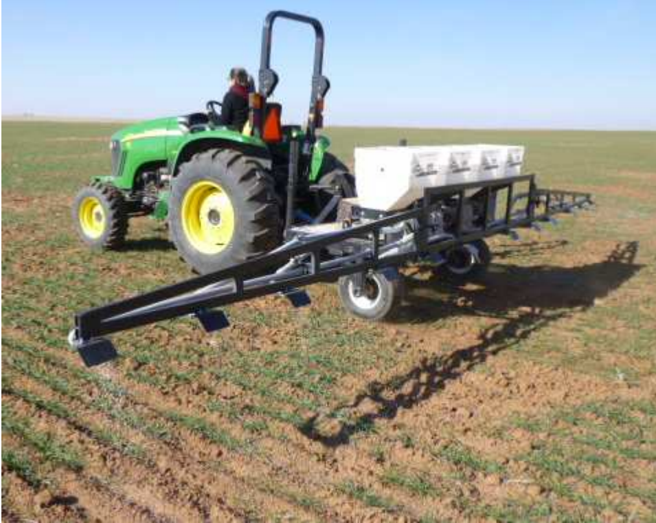
Figure 1. Application of NPKS rich strips with an applicator built by engineers at Oklahoma State University, containing four dry fertilizer boxes that held individual fertilizer connected to three polyvinyl chloride tubes attached to a 12 m boom. Fertilizer boxes were fed by two drive wheels as a PTO controlled fan forced fertilizer through the polyvinyl tubing to a reflection plate where it was evenly dispersed throughout a 1.8 m strip parallel to one another.
