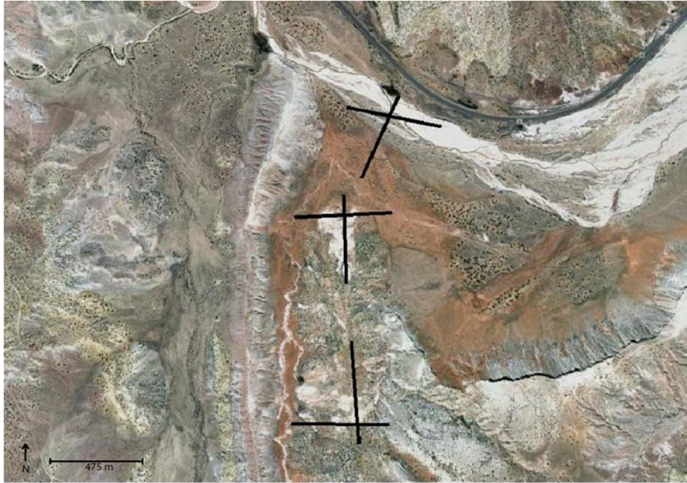
Figure 4.2: Map view of preliminary ERI survey lines collected during May, 2011 (aerial photo from Google Earth, May 5, 2012).
