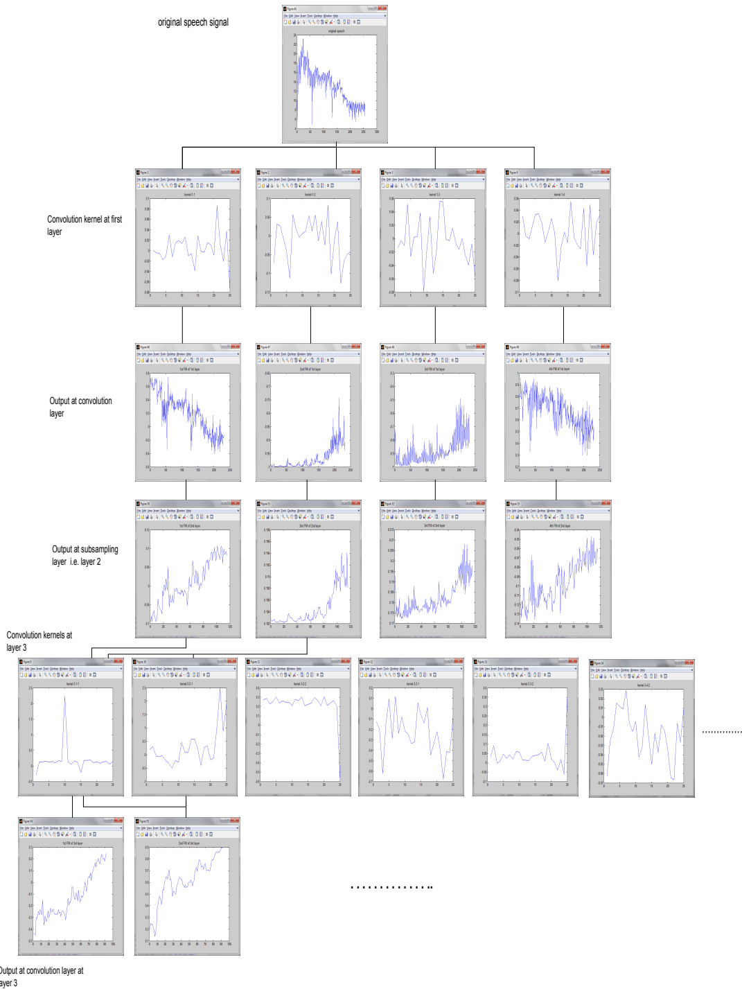
Figure 5.7: Convolution kernels for LeNet-1
