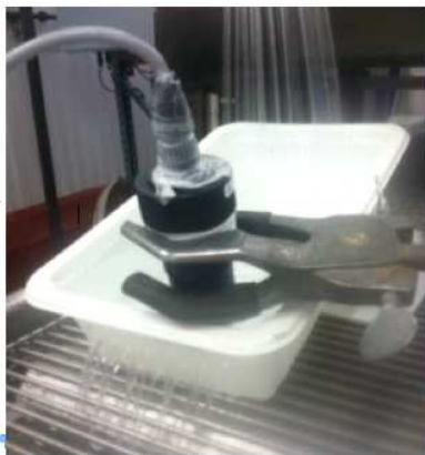
Figure 8. Plastic trough with holes at bottom to allow continuous exit of ozone as it flows into the system.
