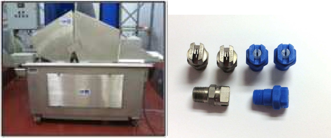
Figure 2. Ross industries spray system. Stainless steel and kynar spray nozzles.
