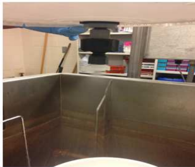
Figure 5. Single nozzle spray utilized in pressurized EW application.
