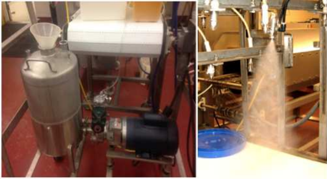
Figure 4. Pump and reservoir utilized in air-assisted automated spray system. Air-assisted spray nozzle.
