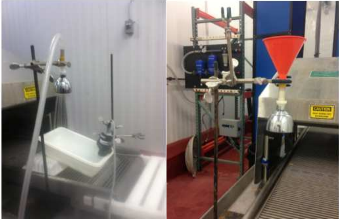
Figure 3. Delta showerhead connected directly to ozone generator (left) and Delta showerhead gravity deluge (right).
