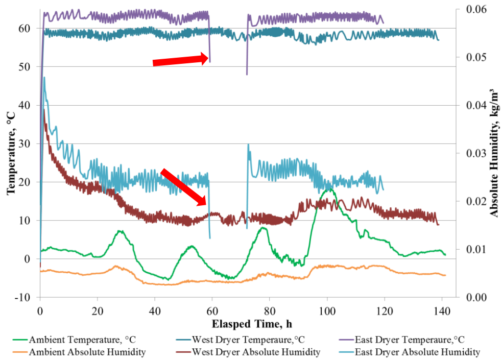
Figure 47. Dryer and ambient temperature and absolute humidity data recorded during drying set one.
