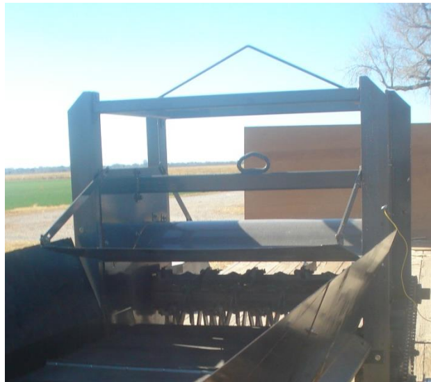
Figure 17. Material guidance shield for the impeller conditioners.
