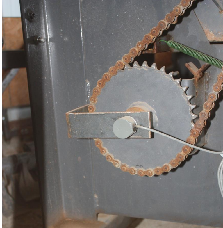
Figure 19. Motor encoder on drive sprocket powering the rollers and rotors.
