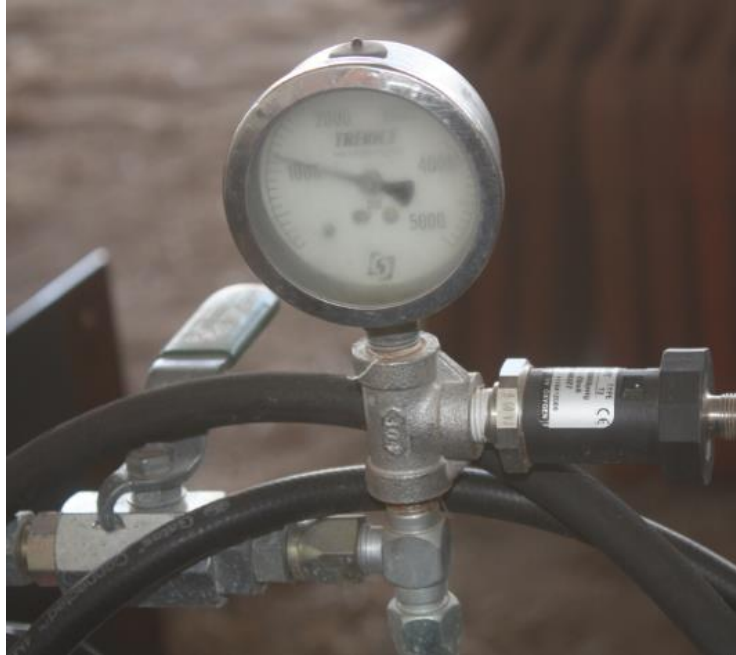
Figure 20. Roll-to-roll pressure transducer and readout gauge for the fluted conditioner.
