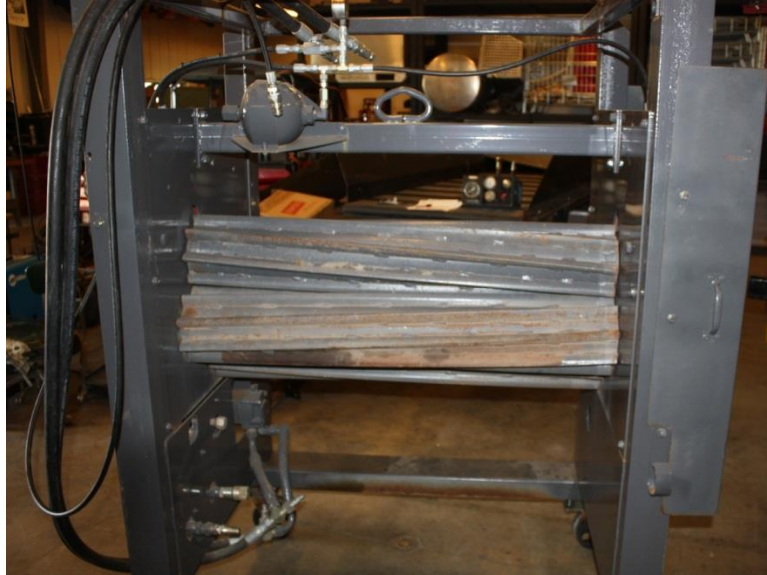
Figure 10. Fluted roll conditioner unit.
