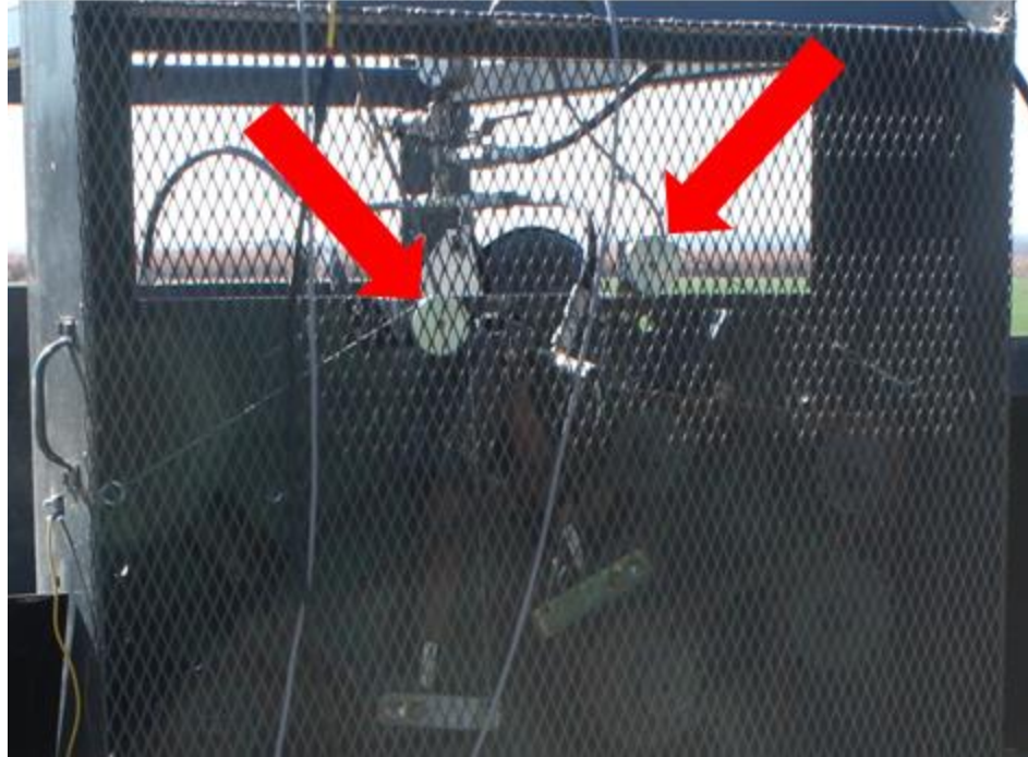
Figure 21. Potentiometer sensor arrangement that monitors roller movement for the fluted conditioner.
