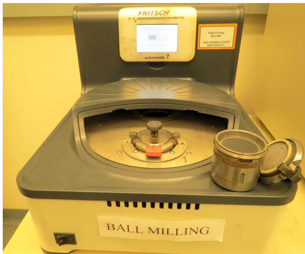
Figure 2.2 High energy planetary ball mill.
