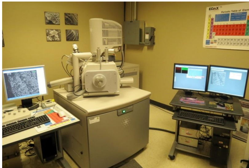
Figure 2.10 Energy dispersive x-ray spectroscope.
