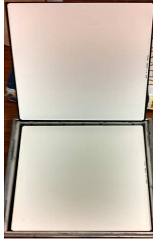
Figure 2-5: A typical cassette composed of two intensifying screens inside of a light-tight container. The film is inserted between the screens and closed. The x-rays penetrate the cassette, strike the intensifying screens, and are collected onto the film by way of visible light from the screens.
