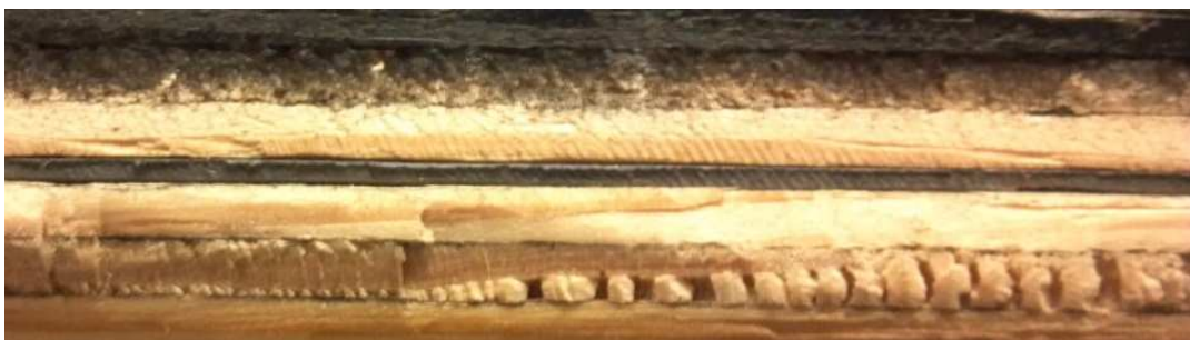
Figure 3-5: The lead was sandwiched between two wooden panels for the lid.
