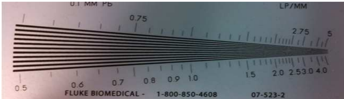
Figure 3-14: A fan-like line pair phantom that has the boundaries of 0.5-5 LP/mm.
