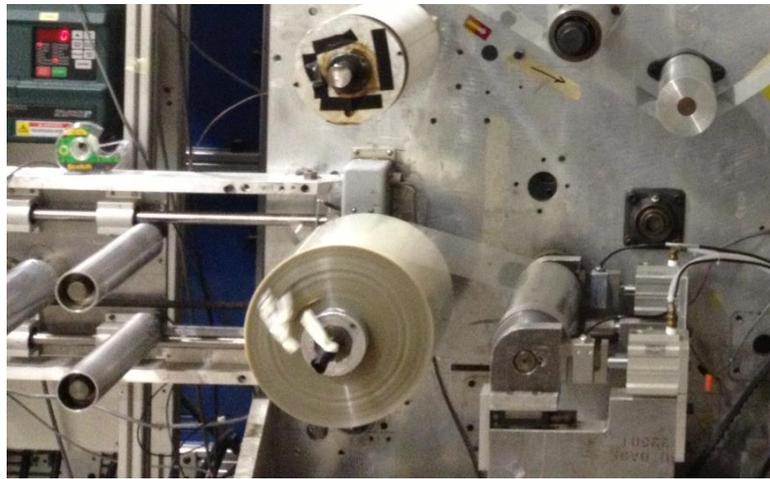
**Figure 4.10 : Wound roll with Pull Tabs inserted at specific radii.**
