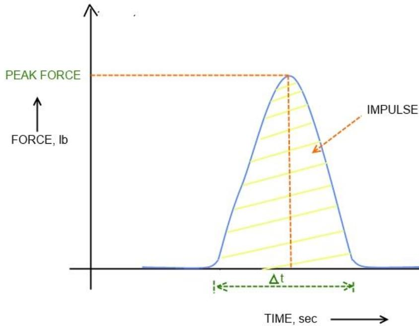
**Figure 5.7 : Representation of the Force vs. Time plot during the impact of the striker with the surface of the wound roll.**
