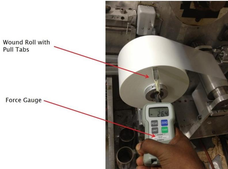
**Figure 4.11 : Pull Tab test on a wound roll.**
