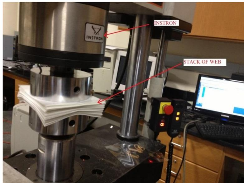
**Figure 4.3 : Stack Compression Test on INSTRON.**
