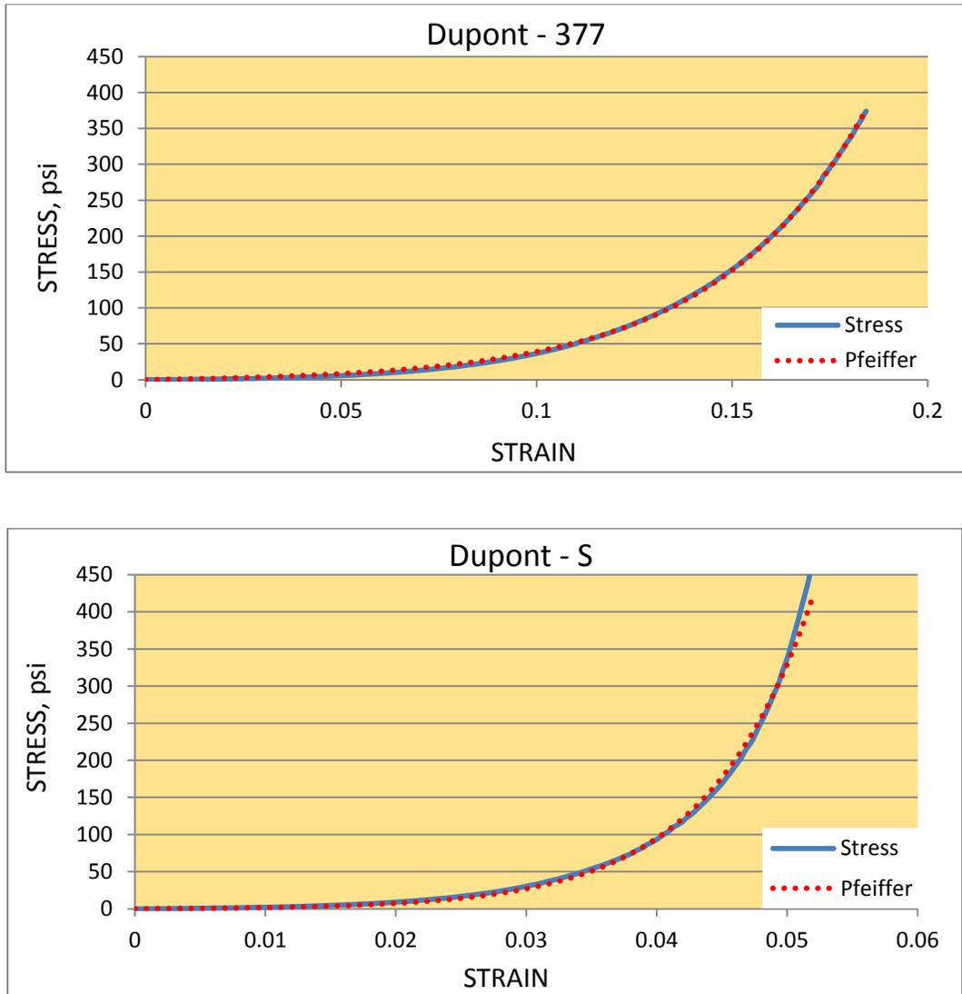
**Figure 4.4 : Stress vs. Strain plots of Dupont-377 and Dupont-S.**
