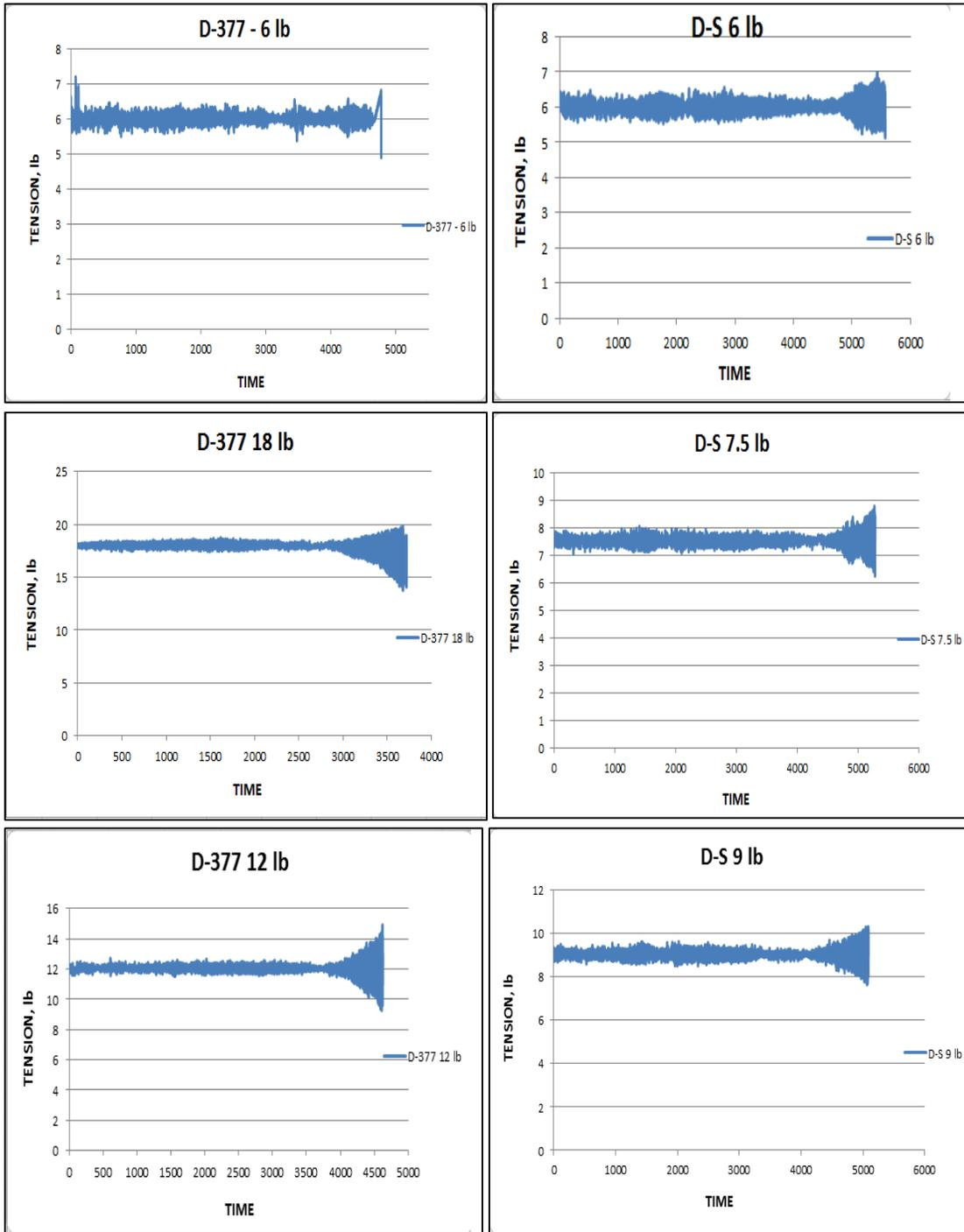
**Figure 7.2 : Tension vs. Time plots during winding the rolls of the two materials.**
