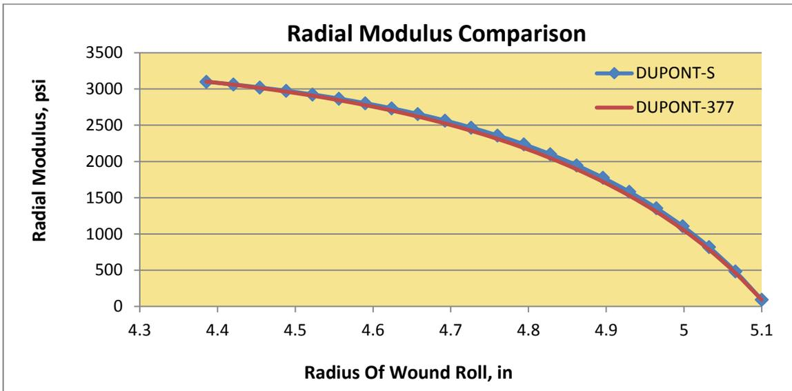
**Figure 5.8 : Radial Modulus of Dupont–377 and Dupont-S when wound at their respective tensions of 13.45 lb and 3 lb.**
