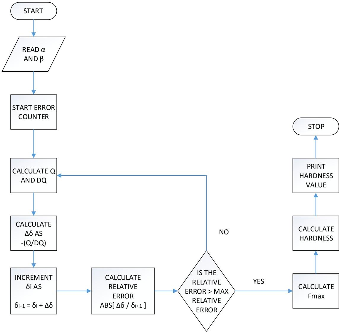
**Figure 6.6 : Flow chart explaining the working of the 1-D Hardness Predictor Algorithm.**
