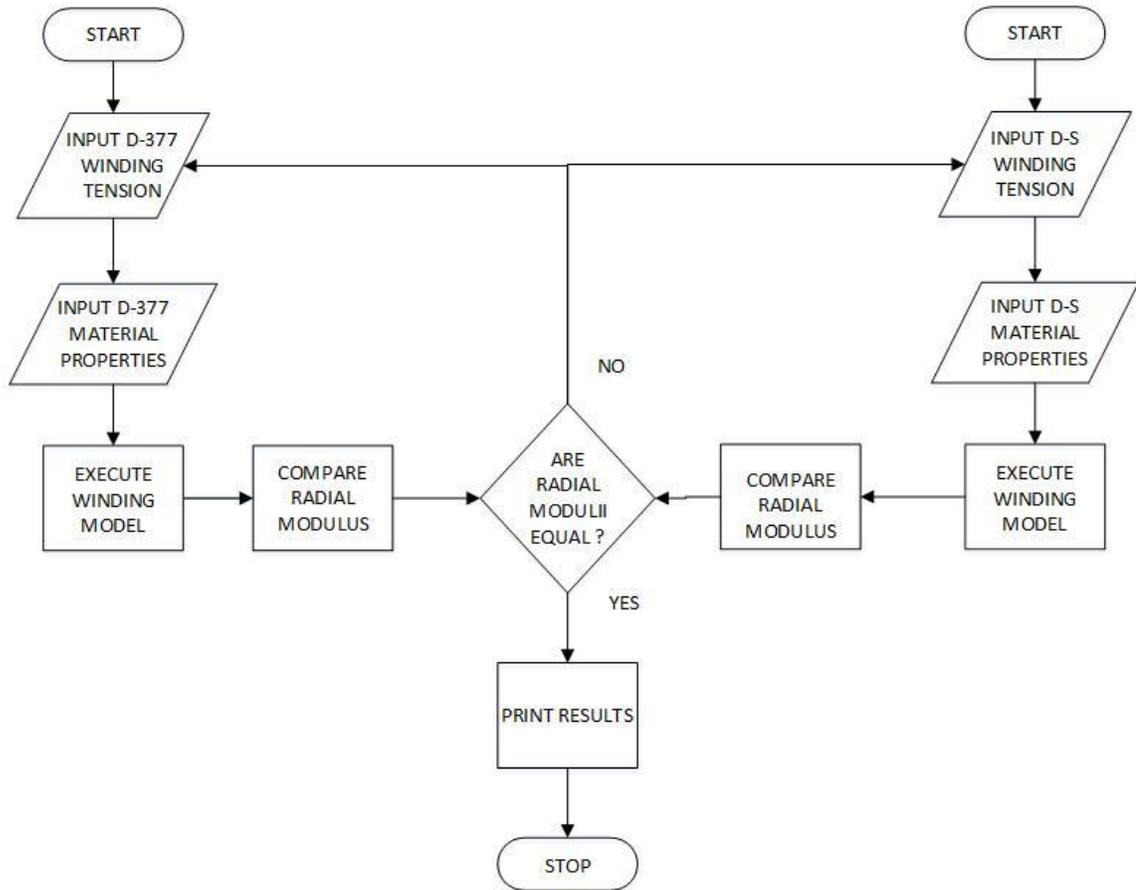
**Figure 5.3 : Flow chart to obtain winding tensions for Dupont-377 and Dupont-S with the criterion of equal radial modulus.**
