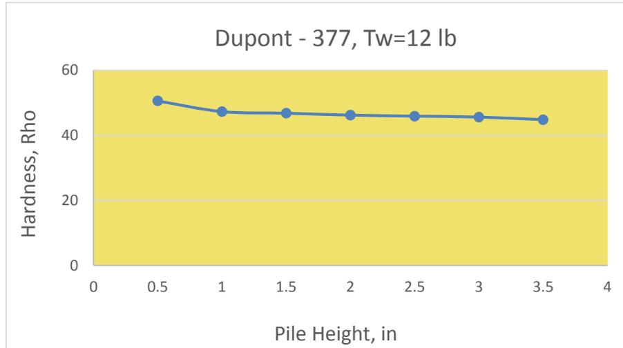
**Figure 7.6 : Plot showing hardness variation with increase in pile height of a roll.**
