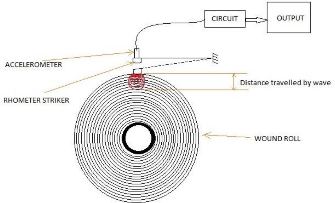
**Figure 5.5 : Figure showing the depth of wave travel at the instant of hardness measurement using a Rho Meter.**
