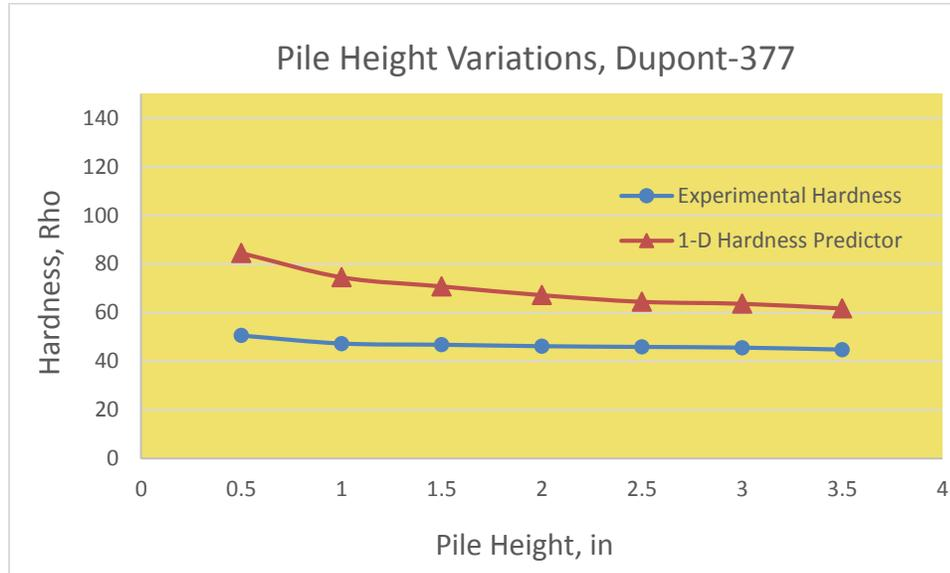
**Figure 7.7 : Plot showing the comparison between the experimentally obtained hardness values and the values obtained from the code for varying pile height for Dupont-377 wound at 12 lb of winding tension.**
