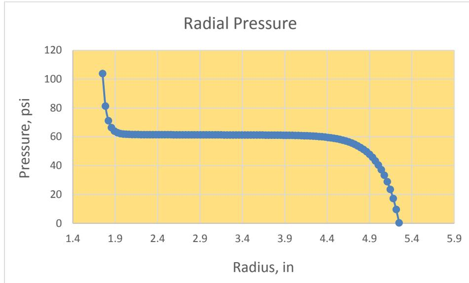
**Figure 5.2 : Sample Pressure profile of a wound roll ( Dupont – 377), 92 gage wound at 9lb.**
