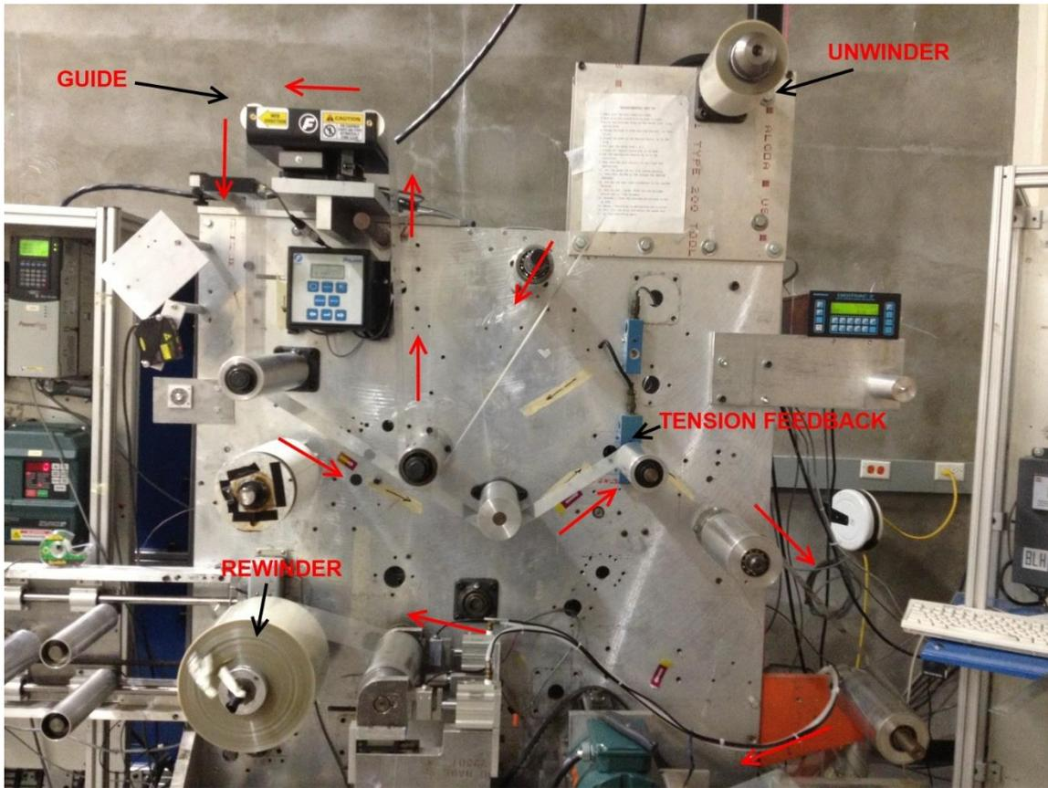
**Figure 7.1 : Center Winder Setup.**
