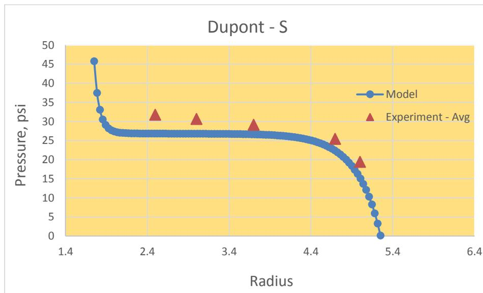
**Figure 4.13 : Pressure vs. Radius plot showing the comparison between experimental and model values for 92 gage DUPONT-S wound at 3 lb tension.**
