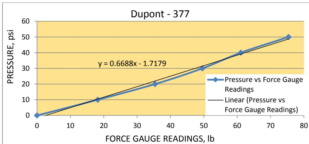
**Figure 4.8 : Pressure vs. Force Gauge Readings plot for Dupont – 377.**
