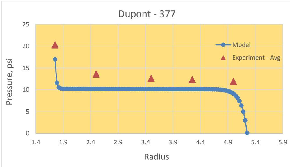
**Figure 4.12 : Pressure vs. Radius plot showing the comparison between experimental and model values for 92 gage DUPONT 377 wound at 3 lb tension.**
