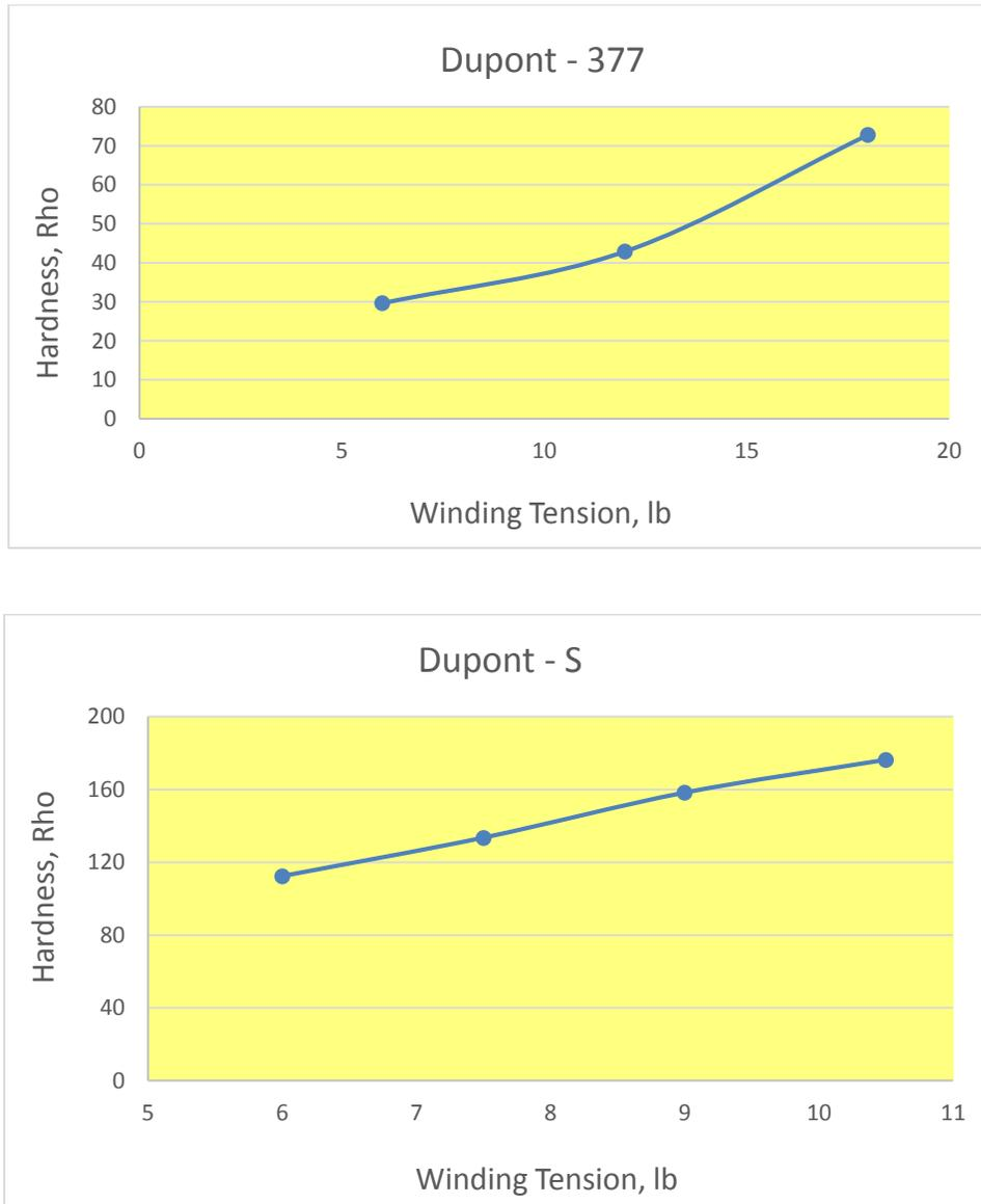
**Figure 7.3 : Plots showing the experimental hardness values of the rolls of each material.**
