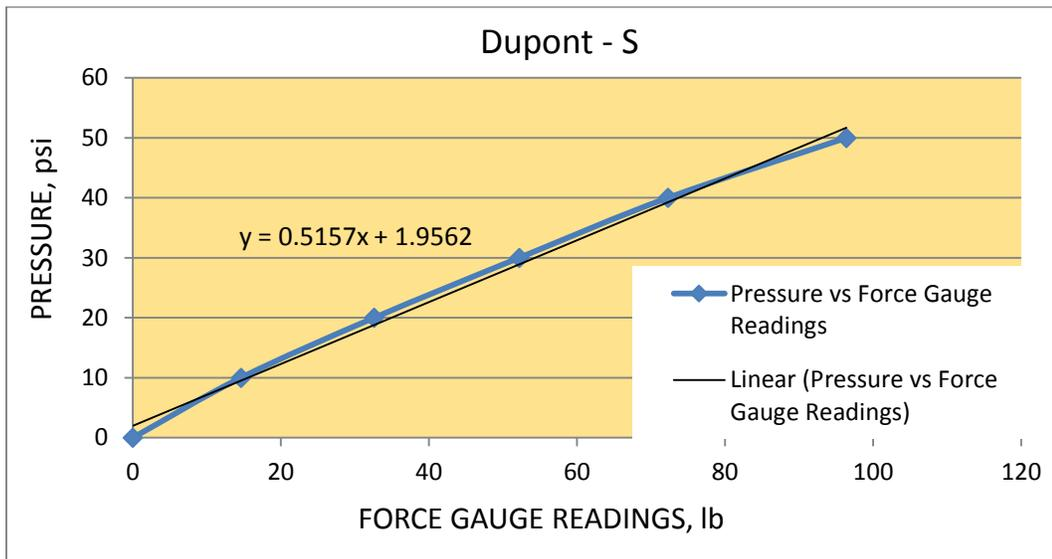
**Figure 4.9 : Pressure vs. Force Gauge Readings plot for Dupont – S.**
