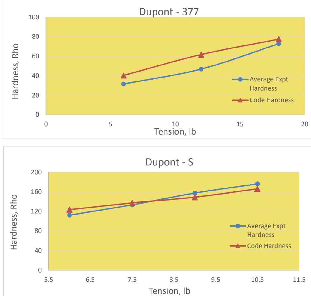
**Figure 7.5 : Plots showing the comparison between the experimental average hardness values and the hardness values obtained from the Hardness Predictor code.**
