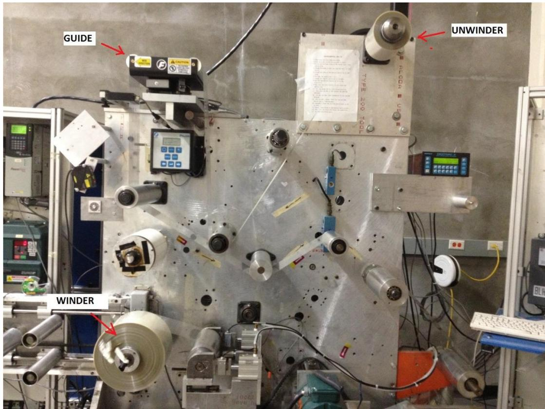
**Figure 4.1 : Small scale winding machine at WHRC, Oklahoma State University.**
