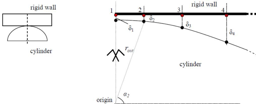
**Figure 6.3 : Geometry of the Node to Node contact of a Rigid Wall and Wound Roll [1].**
