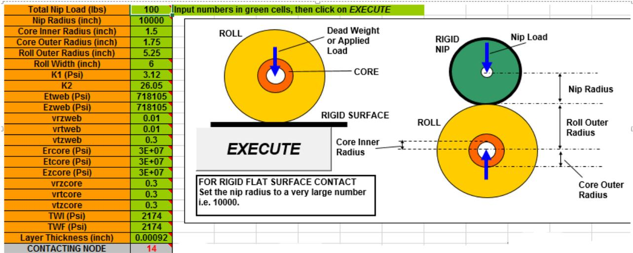
Figure 6.4 : Input interface of the *Roll Compressor*.
