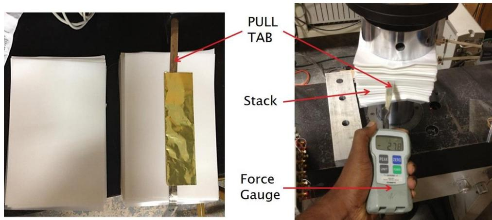
**Figure 4.7 : Pull Tab test.**
