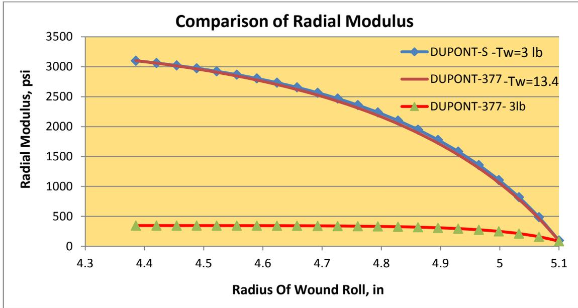
**Figure 5.10: Comparison of radial modulus when Dupont-377 winding tension is equal to 3lb.**
