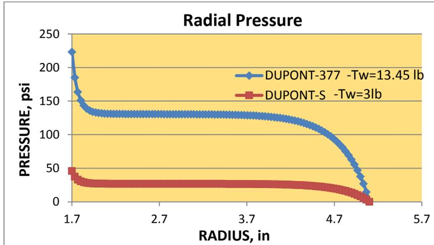
**Figure 5.4: Pressure profiles for Dupont-377 and Dupont-S when wound at their respective winding tensions of 13.45 lb and 3 lb respectively.**
