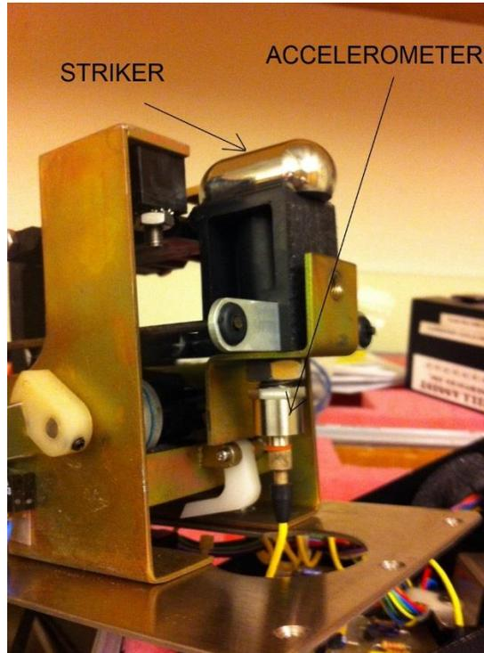
**Figure 6.1 : Striker and Accelerometer of the Rho Meter.**
