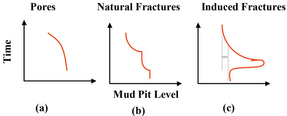
Figure 1.8. Mud loss indication and pit level behavior in pores, natural fracture, and induced fractures.
