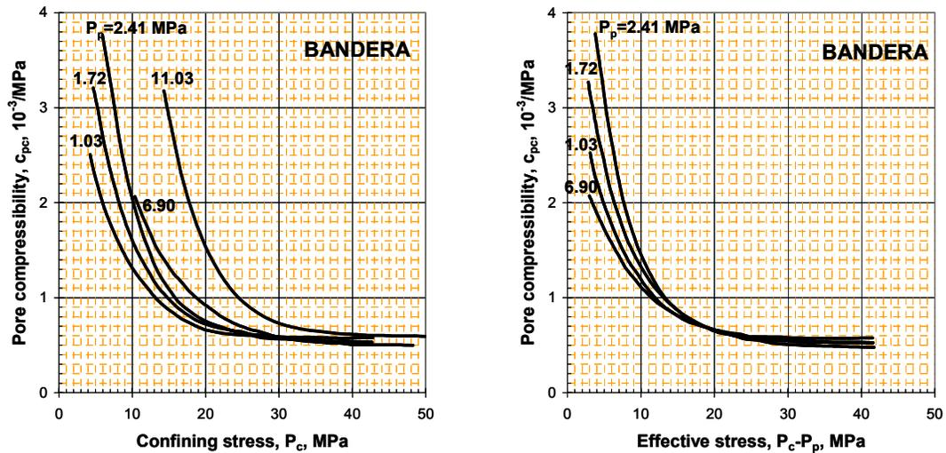
Figure 5.2. Pore compressibility of Bandera sandstone as function of confining pressure and effective stress. (Zimmerman et al.<sup>29</sup>)
