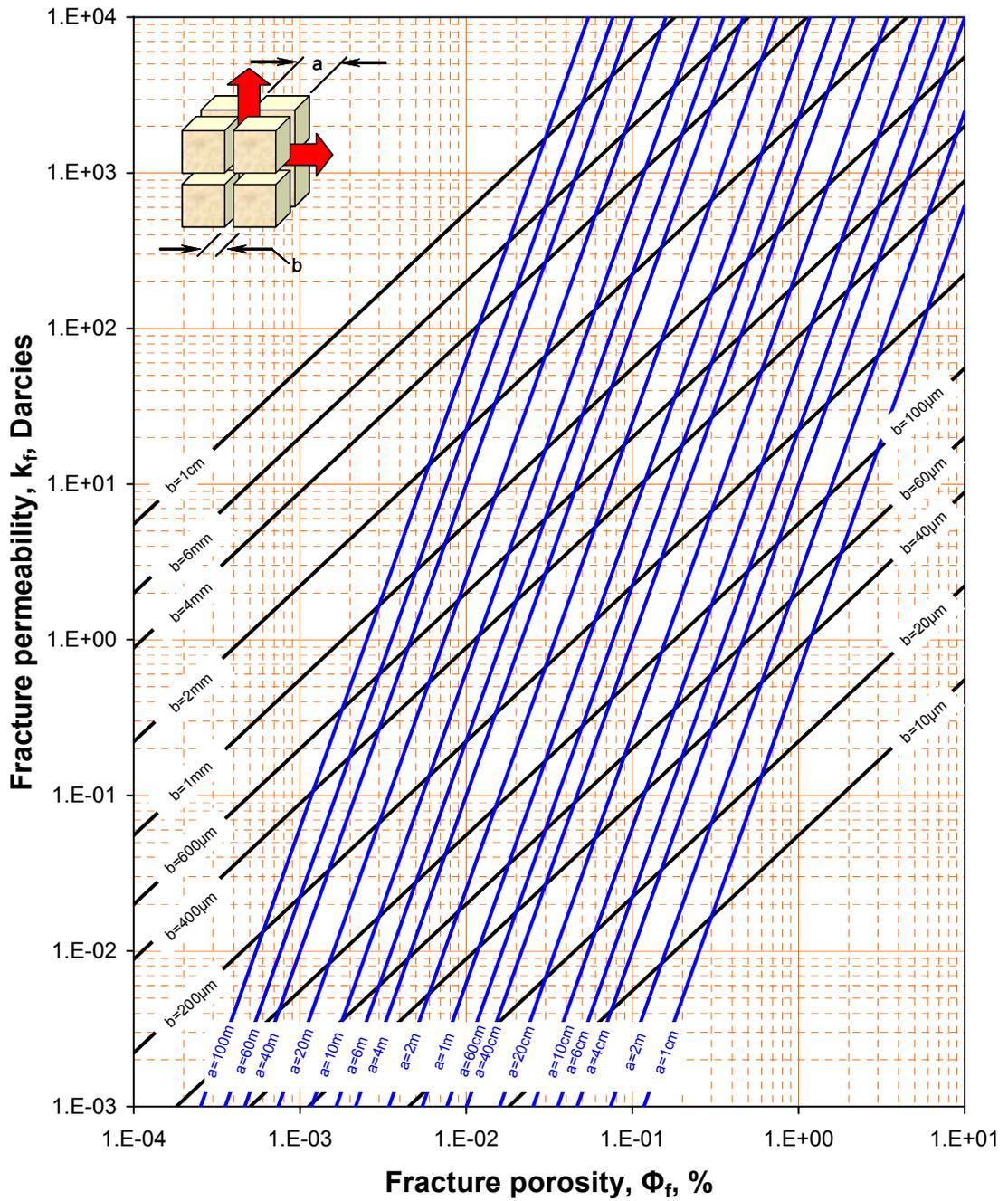
Figure B.0.1. Relationships among fracture permeability  $k_f$ , fracture porosity  $\phi_f$ , fracture width  $b$ , and matrix size  $a$  for the sugar cube model. (After Reiss<sup>8</sup>)
