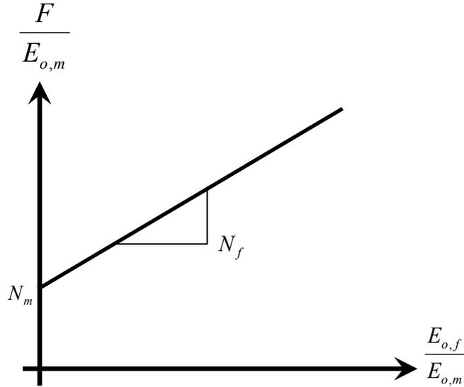
Figure 7.8. Material balance plotting scheme proposed by Penuela et al. (Reference 37)
