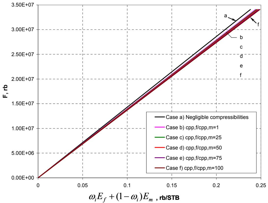
Figure 7.12. Material balance as function of storage capacity ratio for the volumetric saturated NFR example.
