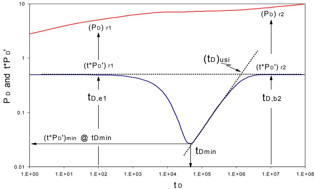
*Figure 4.5. Characteristic lines and points of a naturally fractured reservoir with pseudosteady state interporosity flow  $\omega=0.01$  and  $\lambda=1 \times 10^{-6}$ . (Engler and Tiab<sup>27</sup>)*
