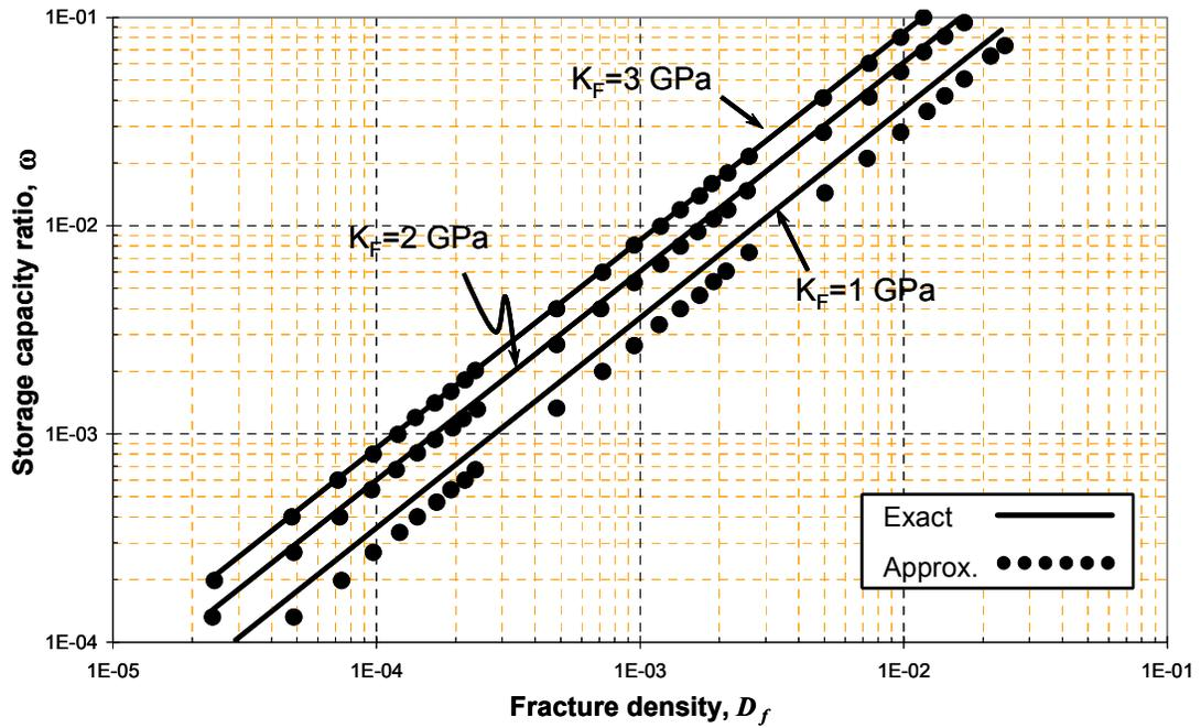
Figure 5.5. Storage capacity ratio vs. fracture density.
