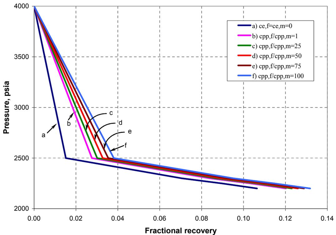
Figure 7.10. Sensitivity analysis on recovery versus pore pressure in an undersaturated NFR.
