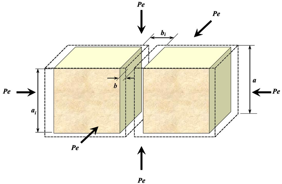
Figure 2.3. Effect of stress on fracture porosity.
