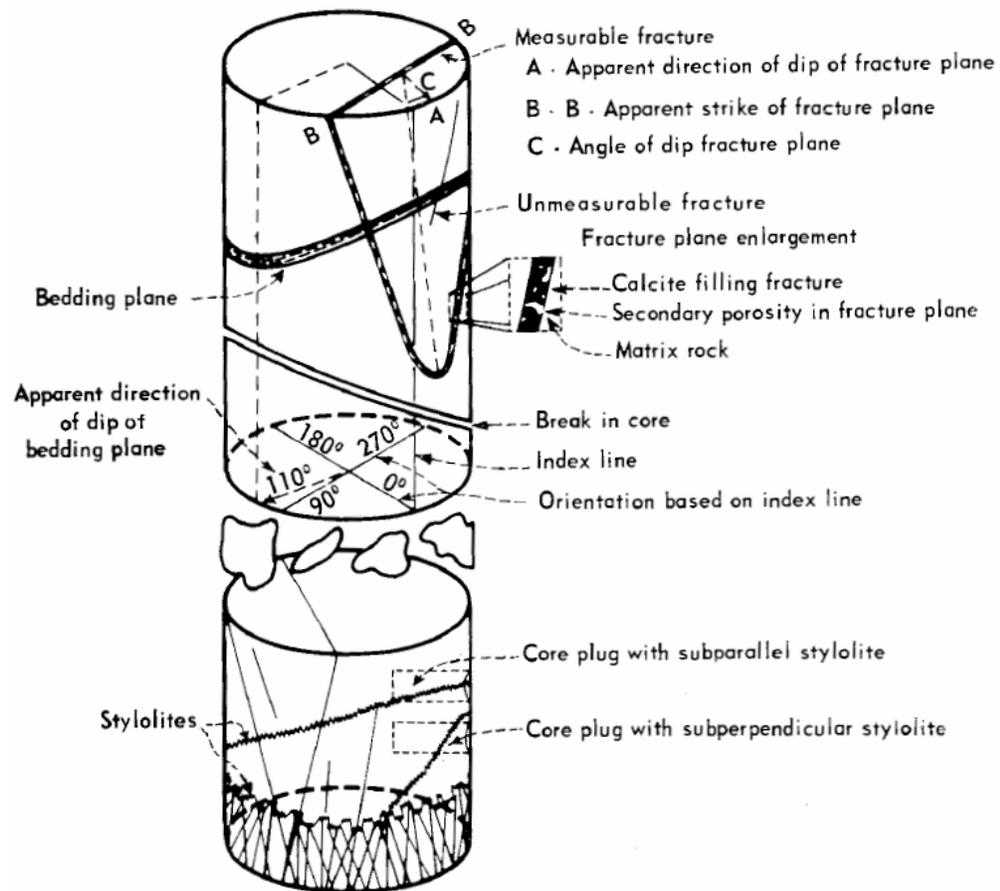
Figure 1.10. Definition of the parameters used to describe cores. (Reis<sup>8</sup>)
