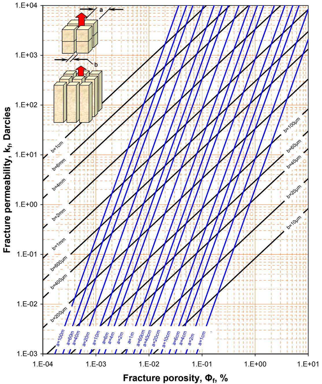
Figure B.0.4. Relationships among fracture permeability  $k_f$ , fracture porosity  $\phi_f$ , fracture width  $b$ , and matrix size  $a$  for matches model with flow parallel to the matches axes. (After Reiss<sup>8</sup>)
