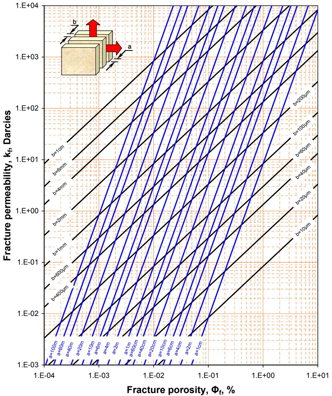
Figure B.0.2. Relationships among fracture permeability  $k_f$ , fracture porosity  $\phi_f$ , fracture width  $b$ , and matrix size  $a$  for the sheets model. (After Reiss<sup>8</sup>)
