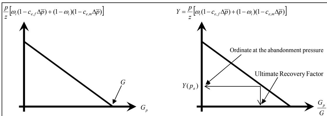
Figure 7.1. Material balance plotting schemes for gas reservoirs.
