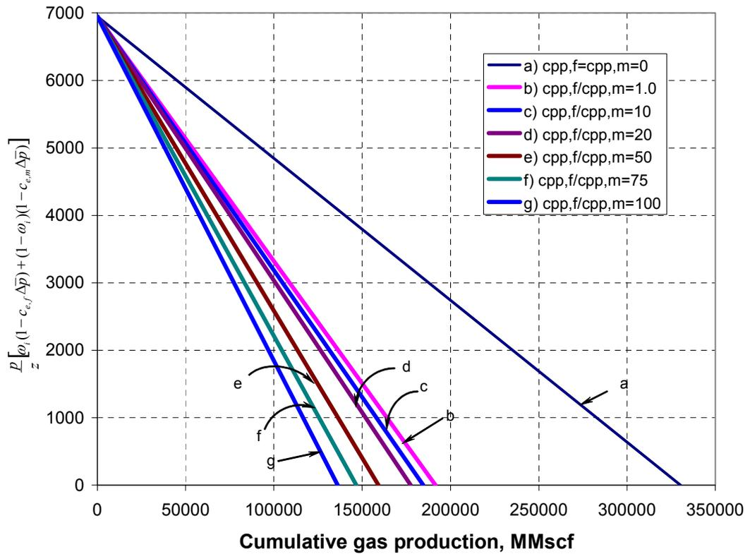
Figure 7.6. Graphical material balance representation for several fracture and matrix compressibility ratios.
