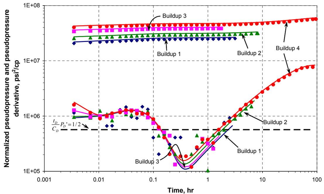
Figure E.0.3. Pseudopressure derivative overlays for the selected pressure buildups.
