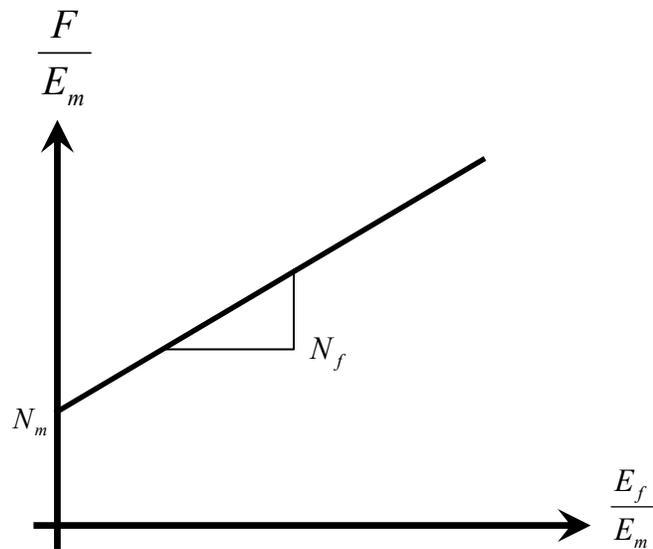
Figure 7.3. Material balance plotting scheme for saturated reservoirs.
