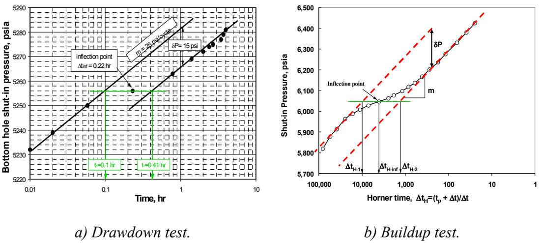
Figure 4.1. Typical pressure curves for a semilog analysis in naturally fractured reservoirs. (Tiab and Donaldson<sup>1</sup>)
