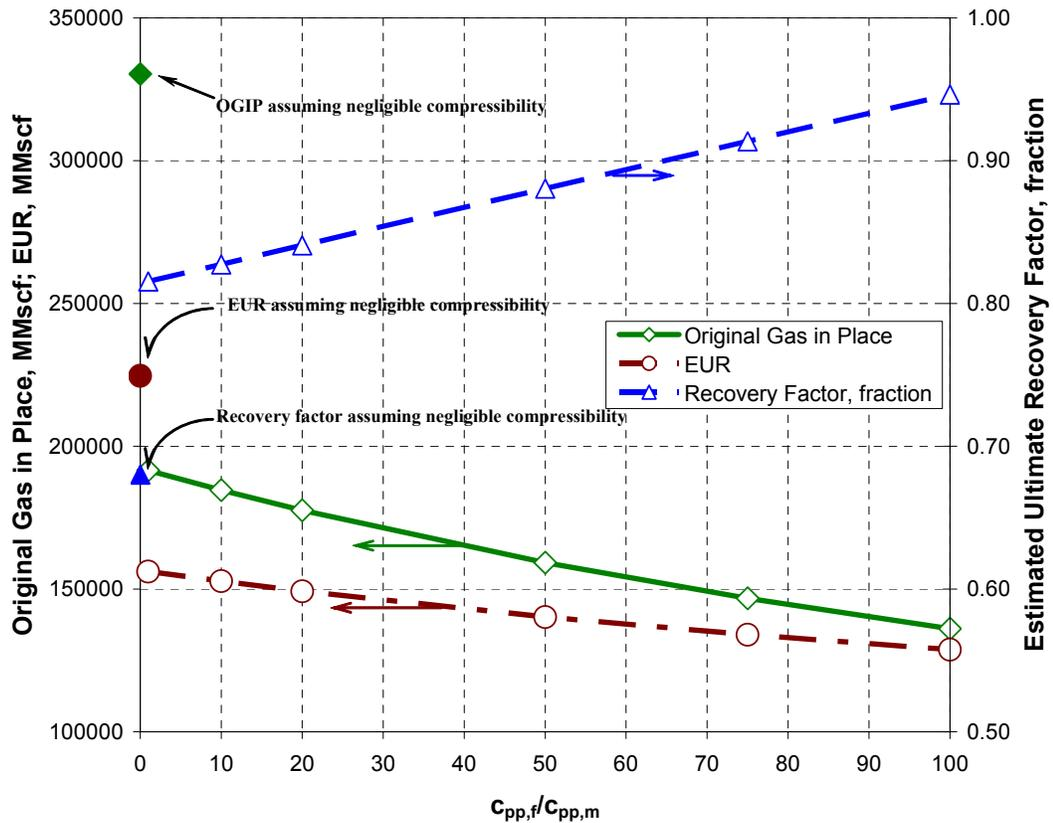
Figure 7.7. Reserves sensitivity to fracture and matrix compressibilities.
