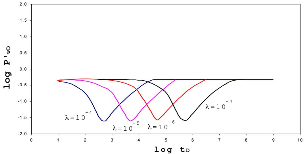
Figure 4.3. Effect of  $\lambda$  on the pressure behavior of dual porosity reservoirs, pseudosteady state model for  $\omega=0.01$ .
