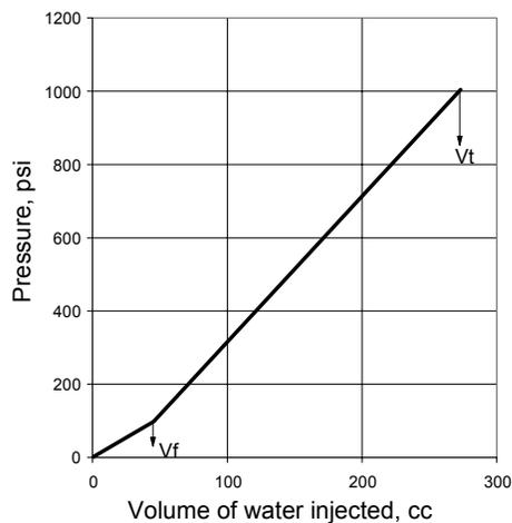
*Figure 2.2. Locke and Bliss method for estimating the fracture pore space. (Tiab and Donaldson<sup>1</sup>)*
