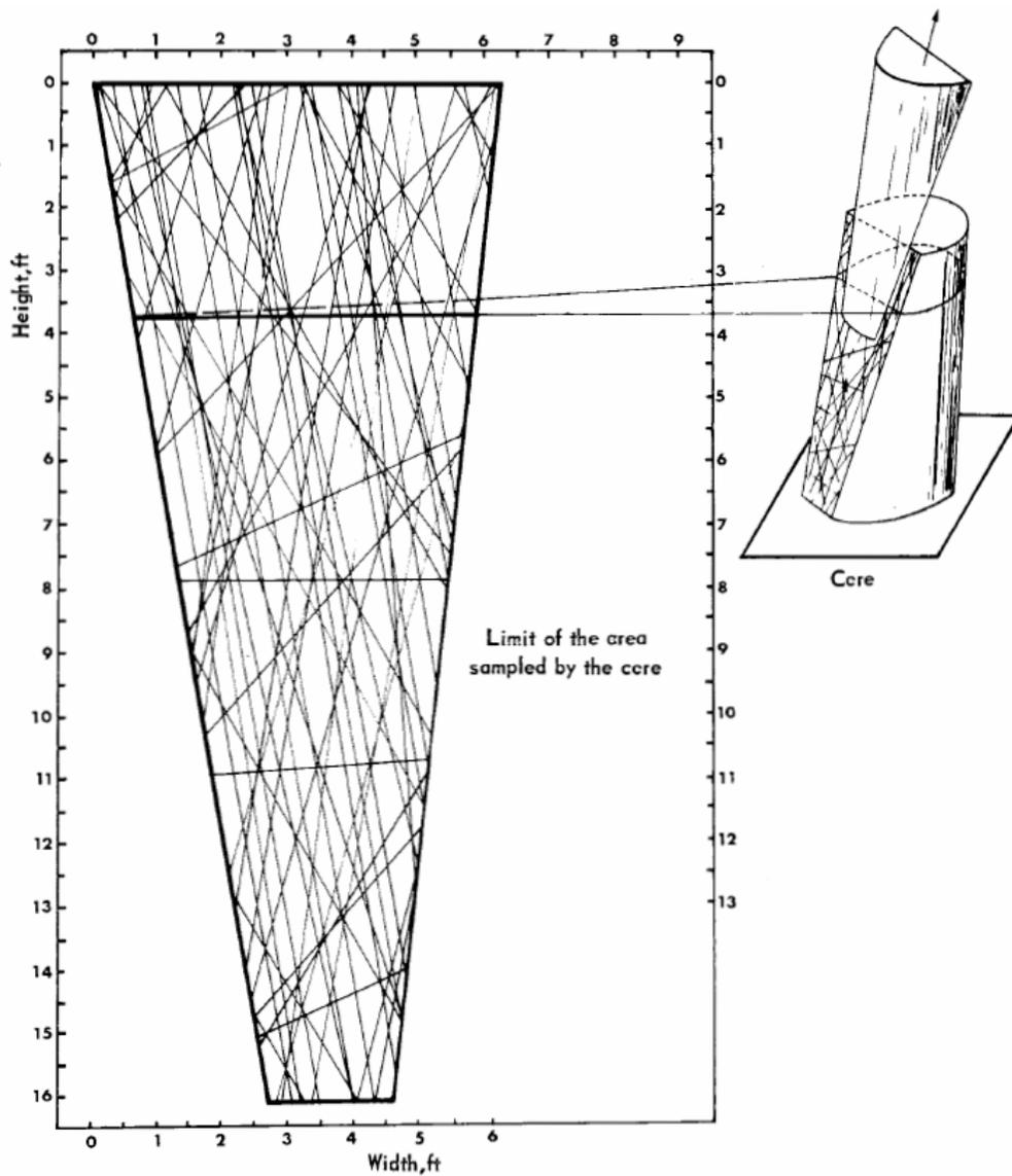
Figure 1.11. Analysis of matrix element size from core description.
