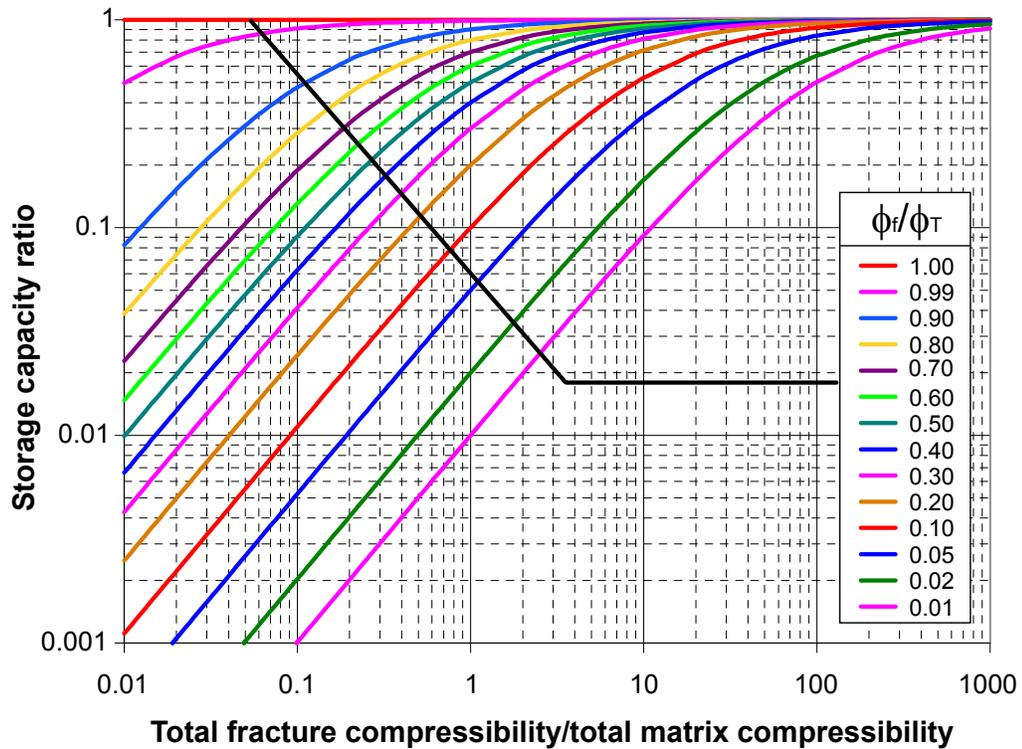
Figure 5.3. Effect of compressibilities on the storage capacity ratio.
