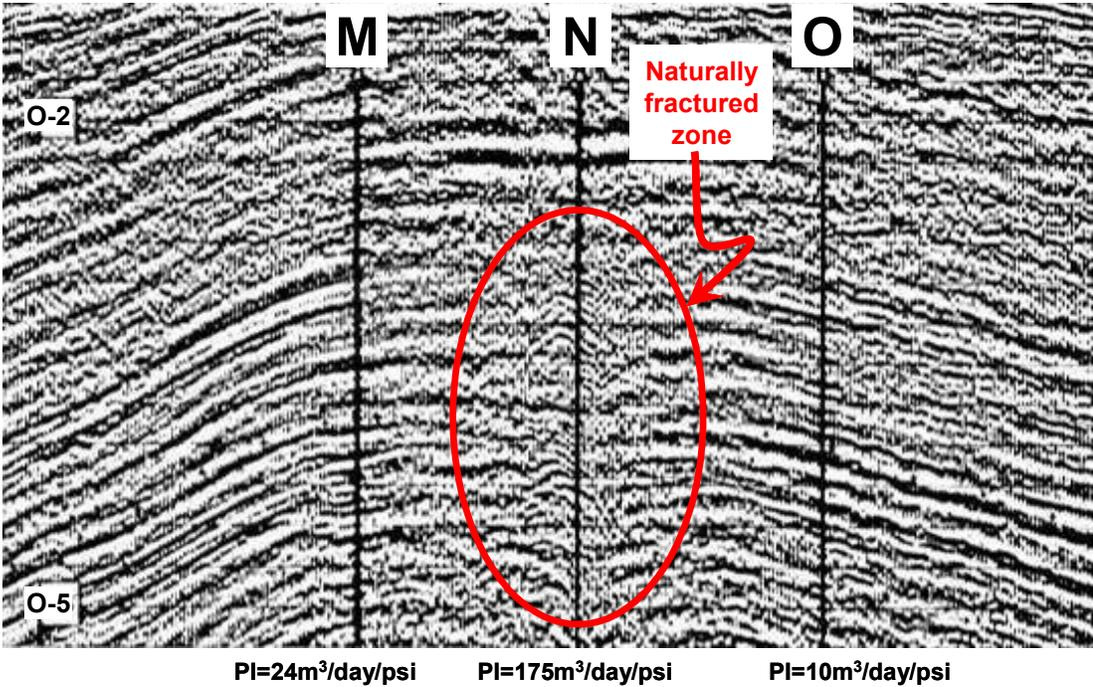
Figure 1.2. Example of seismic profile detecting fractures (Emeraude Field, Congo).
