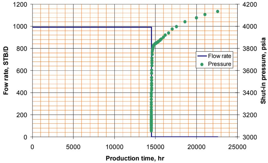
Figure 6.1. Cartesian plot of flow rate and shut-in pressure vs. production time.
