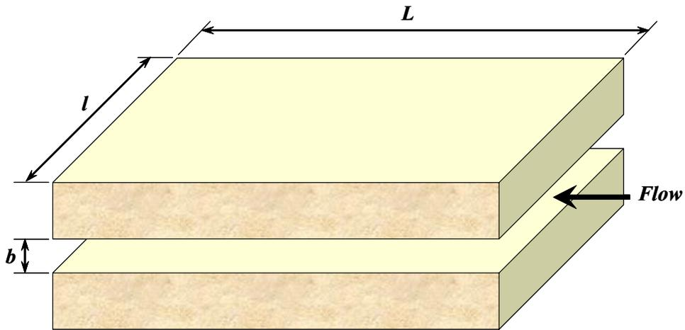
Figure 3.1. Fracture permeability definition.
