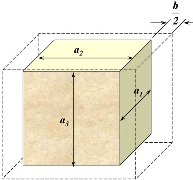
Figure 2.1. Fracture porosity definition.
