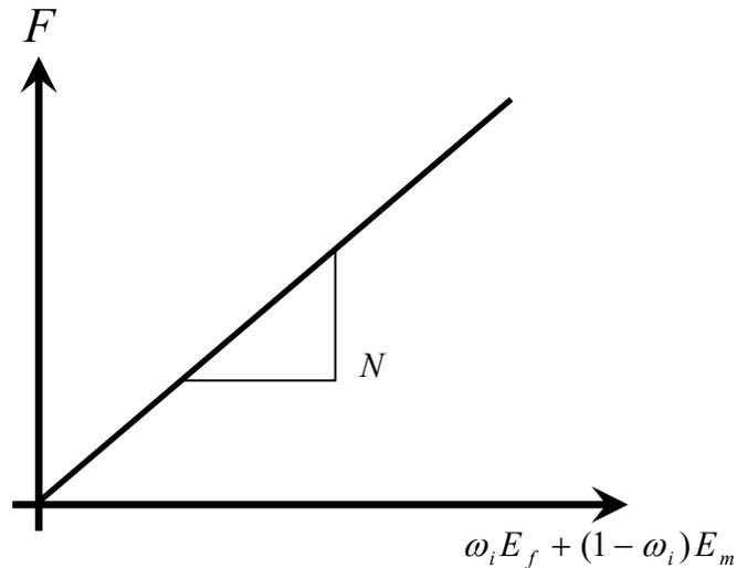
Figure 7.11. Material balance as function of storage capacity ratio for a volumetric saturated NFR.
