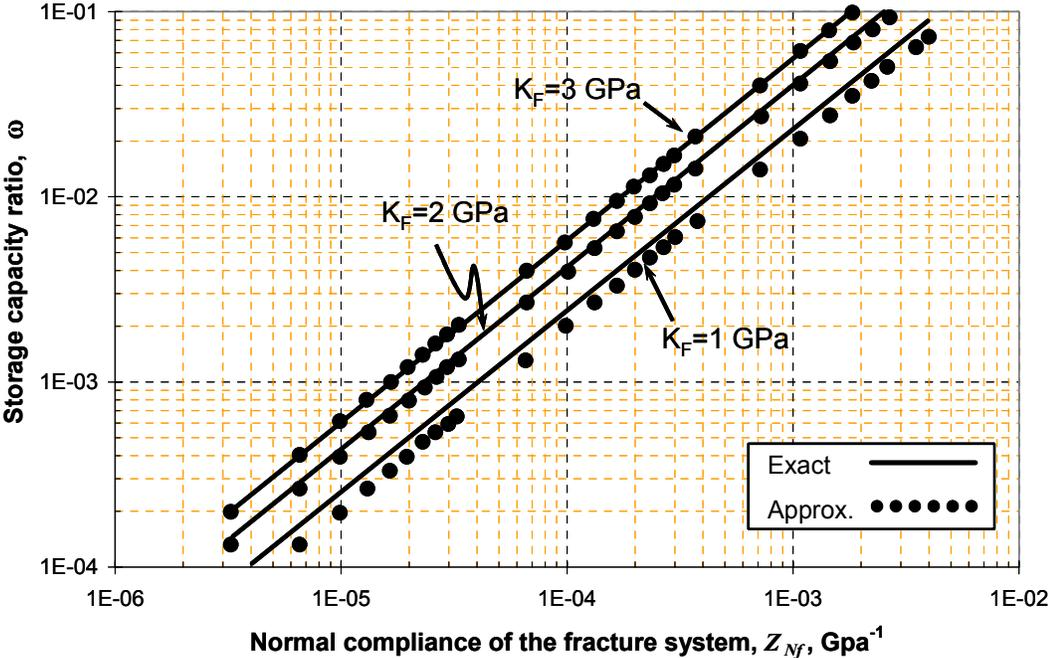
Figure 5.4. Storage capacity ratio vs. normal compliance of the fracture system. (Cardona *et al.*<sup>28</sup>)
