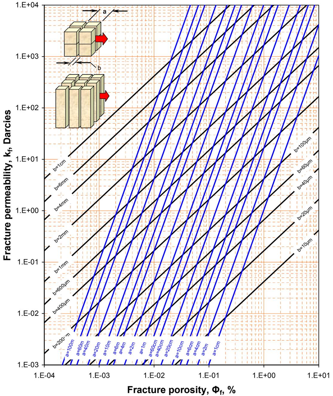
Figure B.0.3. Relationships among fracture permeability  $k_f$ , fracture porosity  $\phi_f$ , fracture width  $b$ , and matrix size  $a$  for matches model with flow perpendicular to the matches axes. (After Reiss<sup>8</sup>)
