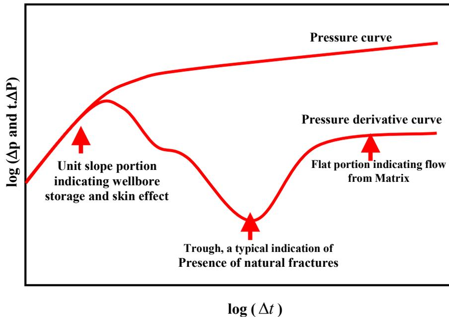
Figure 4.4. Effect of natural fractures on pressure derivative on a log-log plot of pressure and pressure derivative against time.
