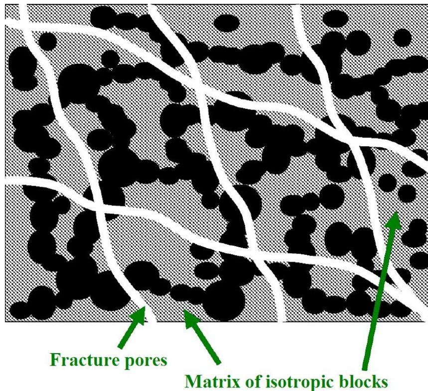
Figure 5.1. Schematic representation of the anisotropic, double porosity rock. (Cardona et al.<sup>28</sup>)
