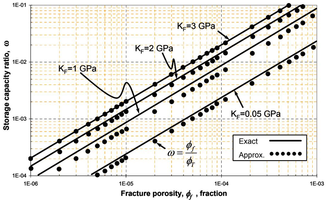
Figure 5.6. Storage capacity ratio vs. fracture porosity.
