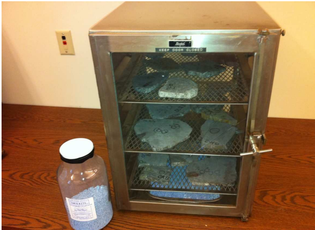
Figure 4-6 The desiccator with anhydrous calcium sulfate crystals
