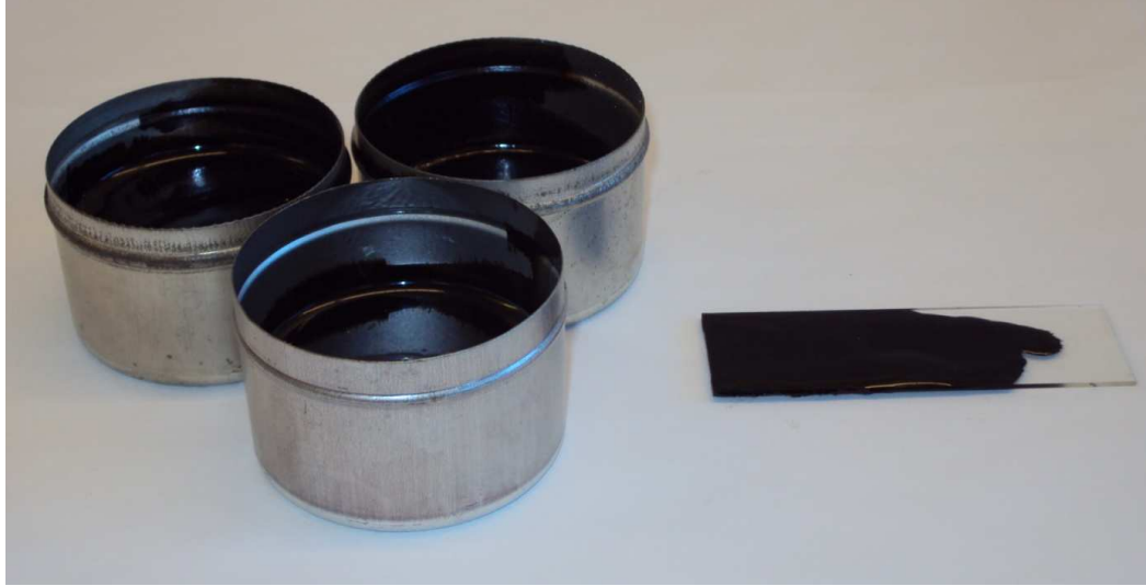
Figure 4-12 PG 64-22 asphalt binder in small canisters and glass slide specimen
