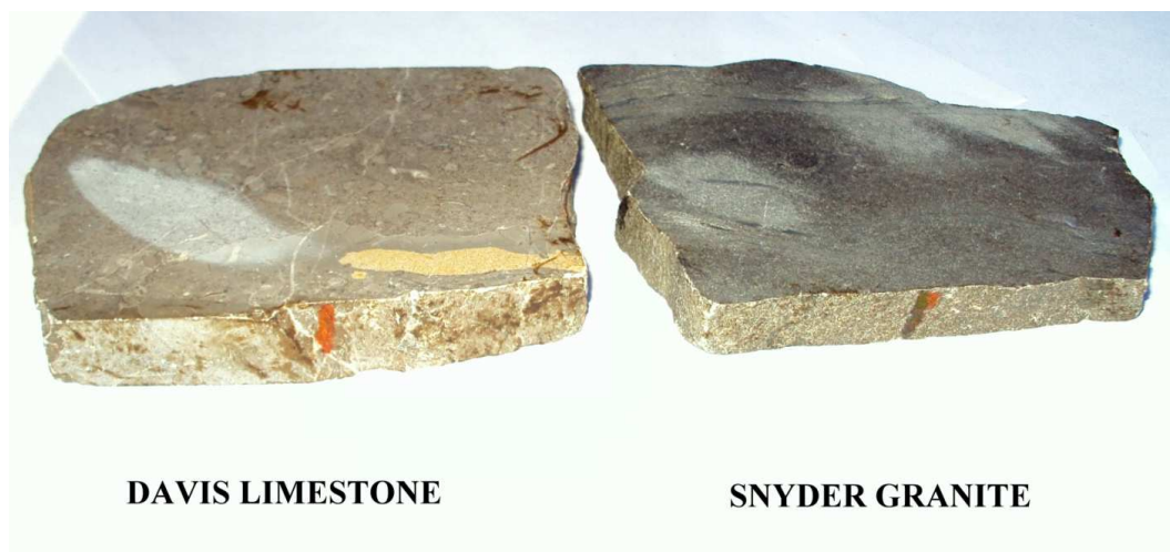
Figure 4-7 Davis limestone and Snyder granite specimens for contact angle measurements
