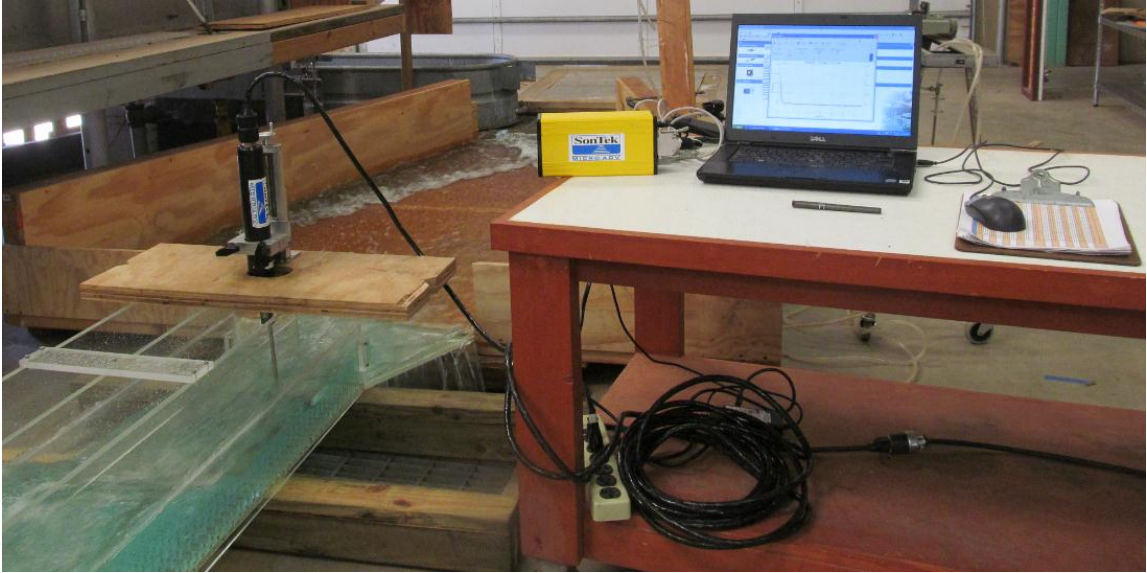
Figure A112: ADV Plugged to Measure the Downstream Velocity V_{d/s}
