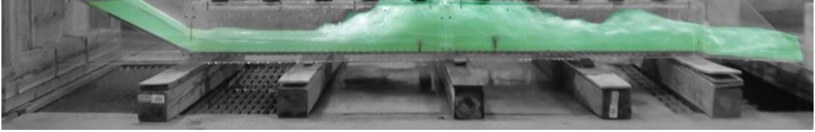
Figure 5.18: Experiment 24A with a 1.5" Sill Located at 37" from the End and a 2" Sill Located at 27" from the End of the Culvert
