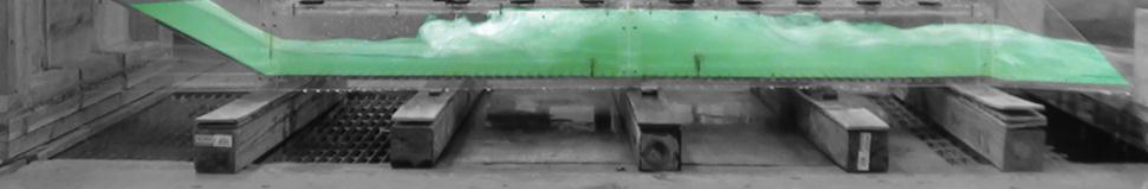
Figure 5.18: Experiment 24A with a 1.5" Sill Located at 37" from the End and a 2" Sill Located at 27" from the End of the Culvert
