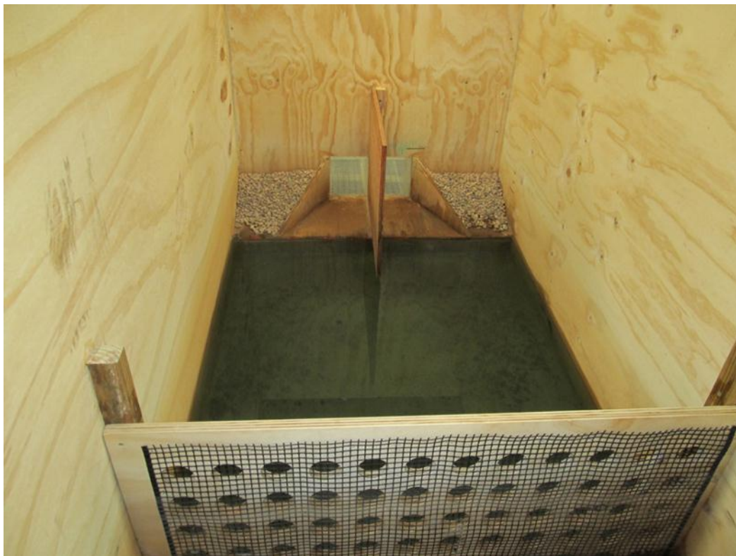
Figure 5.10: Reservoir and Channel Inlet for Culvert Model
