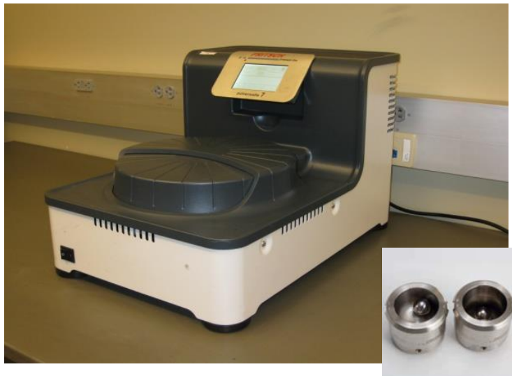
Figure 3-1 Fritsch P7 PL high energy planetary mill with tungsten carbide bowls and balls.
