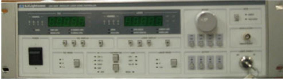
**Figure 2.14:** LDC 3900 diode laser current source with a TEC temperature controller.
