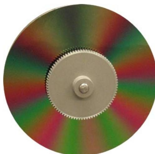
**Figure 2.6:** A front view of circular variable filter wheel in the spectrometer
