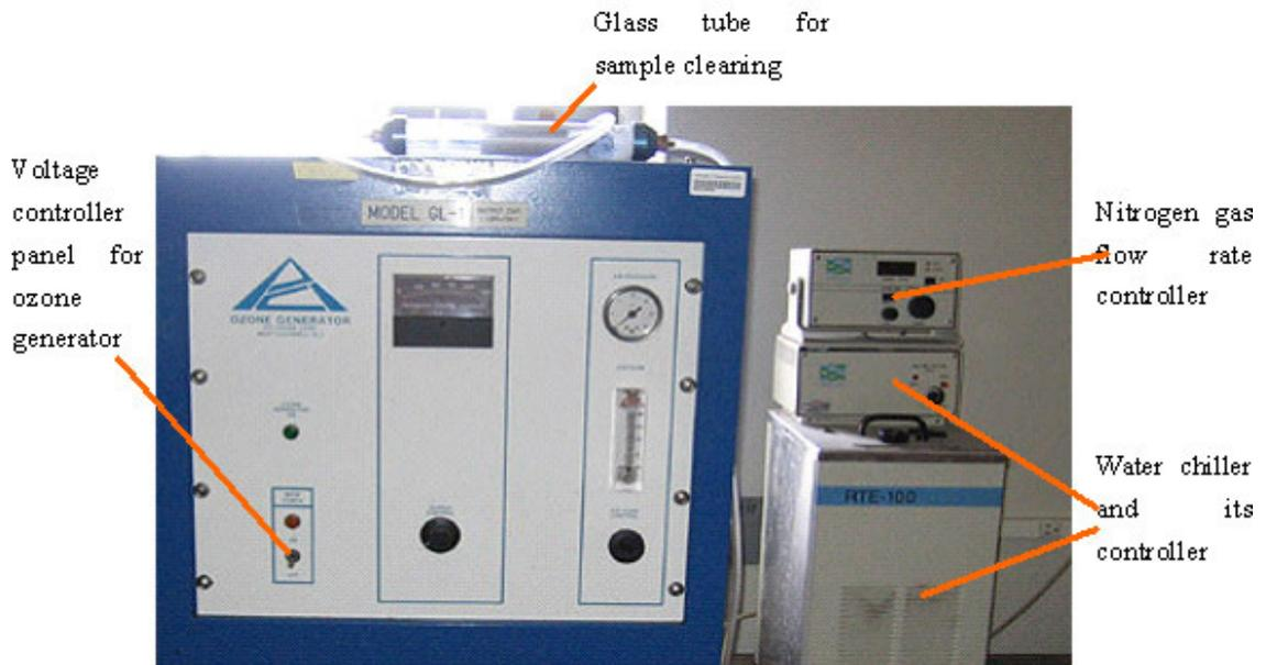
**Figure 3.1:** Picture of Ozone generator (Model GL-1, PCI OZONE CORP)
