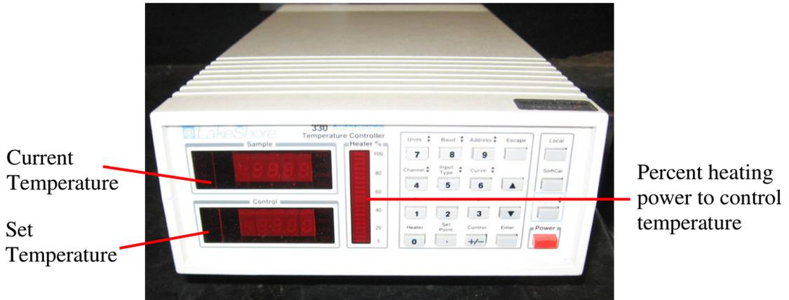
**Figure 4.3:** Front view of a Lakeshore 330 temperature controller
